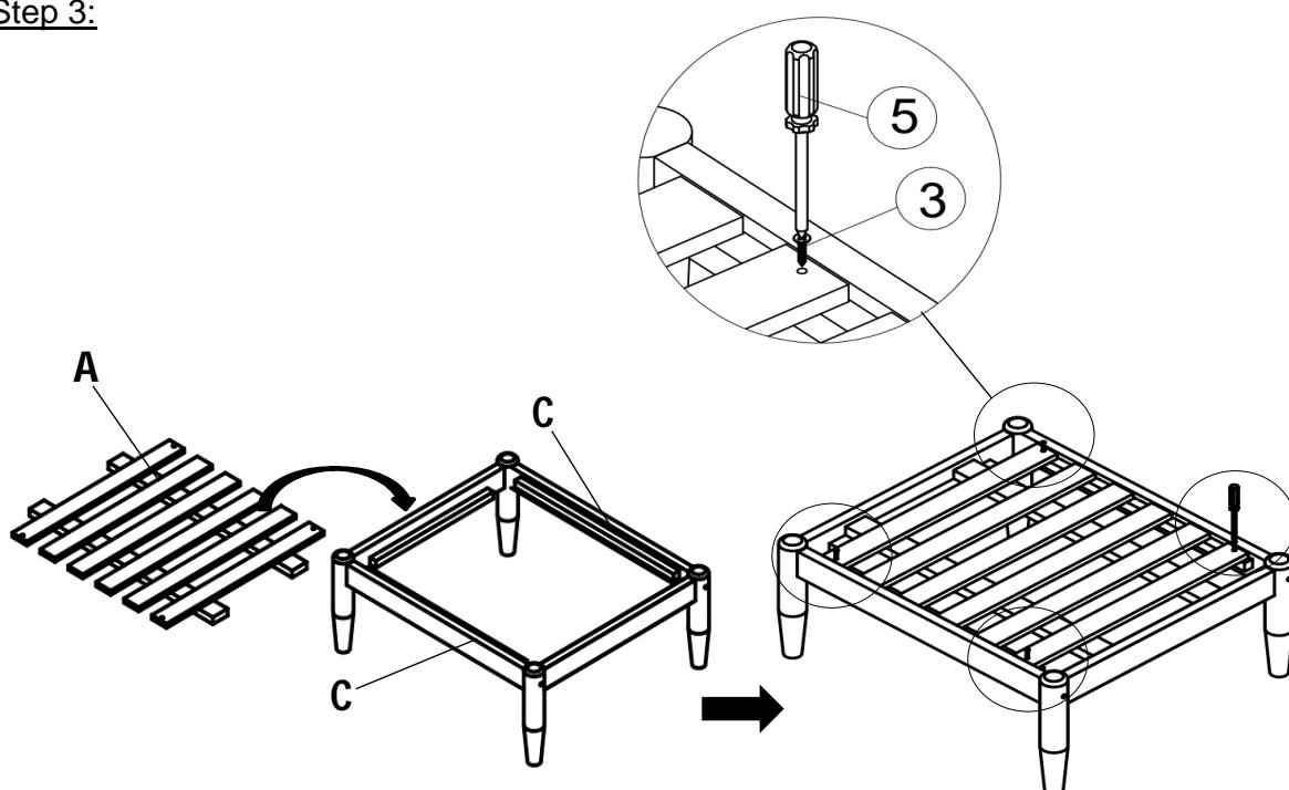
Place the Seat Panel (A) to the assembled part in Step 2 and then secure the Seat Panel (A) to the Support Bars (C) by using Screws (③) and Screwdriver (⑤) as shown above.
