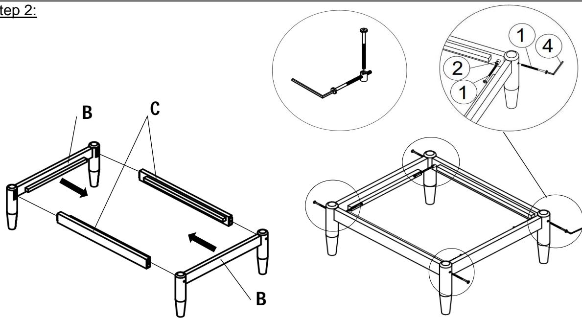
With the help of your adult partner, put the tenons of 2 Support Bars (C) to the mortises of 2 Leg Panels (B) and then secure by using Bolts (①), Nuts (②), Bolt (①) and Allen Wrench (④) as shown in the picture above.
