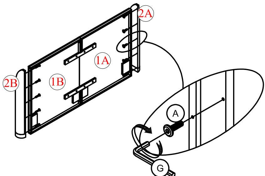
Connect the Headboard to the Left / Right Headboard Side (2A) / (2B) by using 10 Bolts (A) with Allen Wrench (G).
