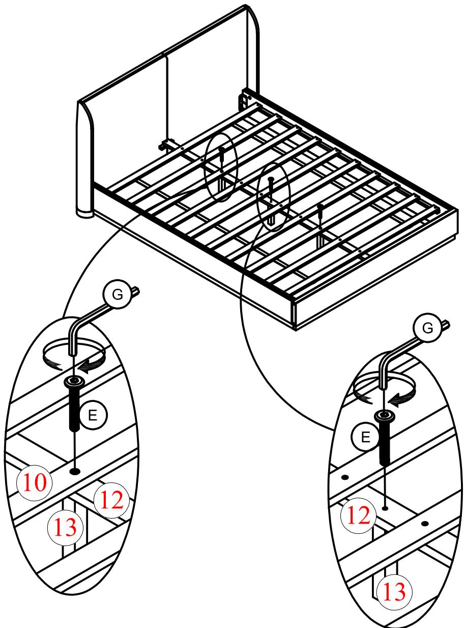
Align the Mounting Position on the Slat Support Bar (12) to the Support Leg (13) and the Slat (10). Attach the Slat (10) and the Slat Support Bar (12) to the Support Leg (13) and by using 3 Bolts (E) with Allen Wrench (G).
