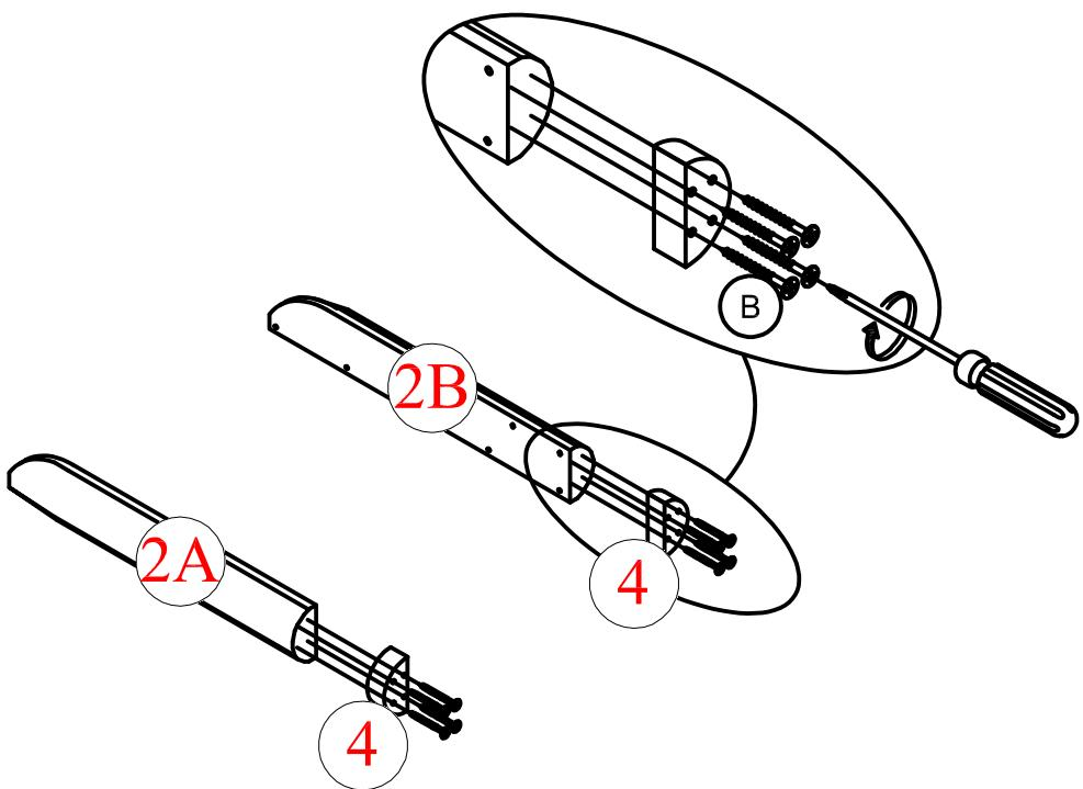
Fix the Bed Legs (4) to the Left / Right Headboard Side (2A) / (2B) by using 8 Screws (B) and a Screwdriver (Not Provided).
