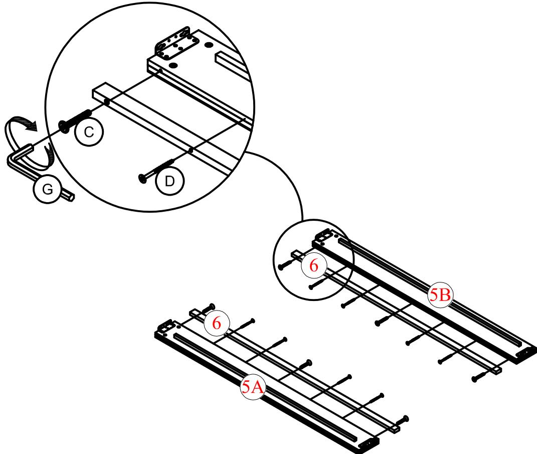
Align the Mounting Position on the Foot Cross Bar (6) to the Left / Right Side Rail (5A) / (5B). Attach the Foot Cross Bar (6) to the Left / Right Side Rail (5A) / (5B) by using 6 Bolts (C), 8 Screws (D) with Allen Wrench (G) and a Screwdriver (Not Provided).
