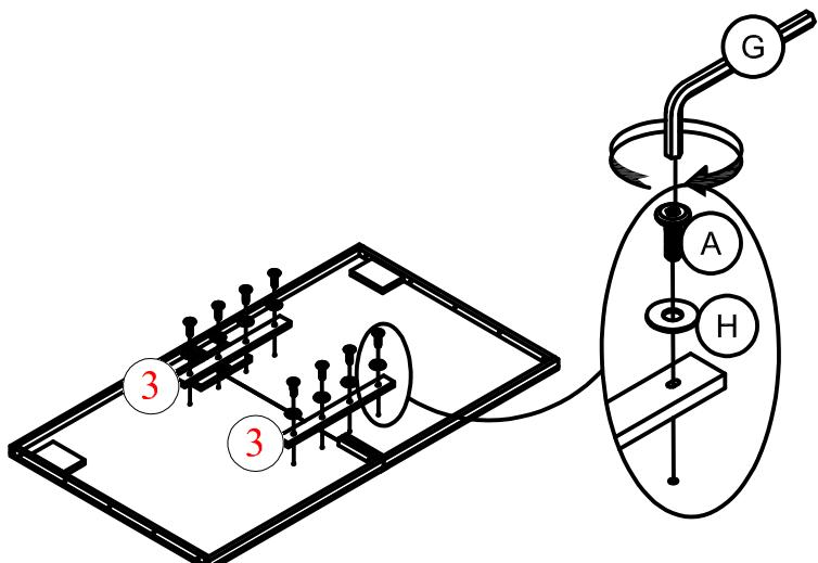
Connect the Crossbar (3) to the Headboard by using 8 Bolts (A), 8 Washer (H) with Allen Wrench (G).
