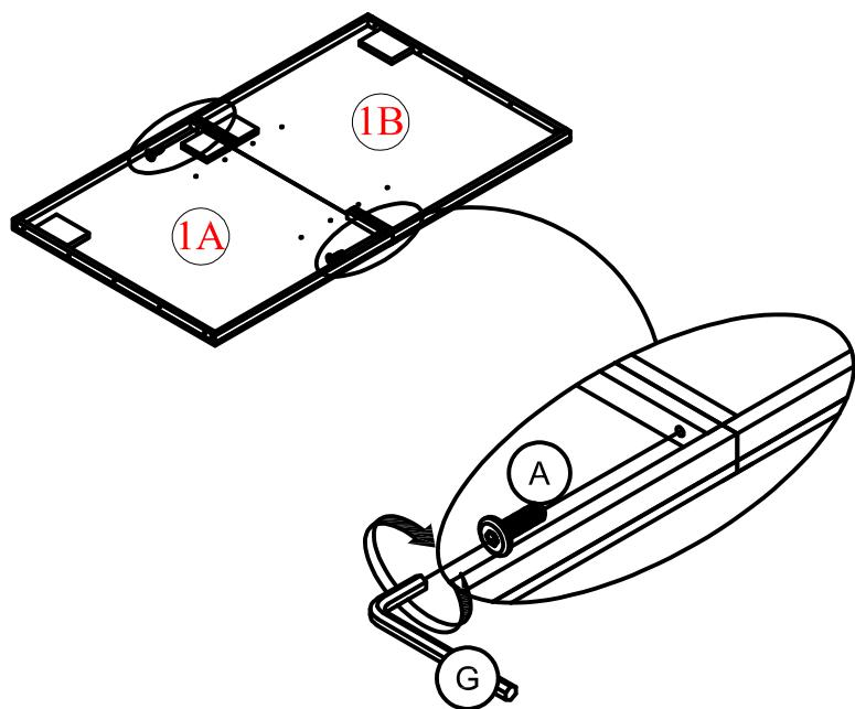
Align the Mounting Position of Left Headboard (1A) into the Right Headboard (1B) as shown above. Affix by using 2 Bolts (A) with Allen Wrench (G).
