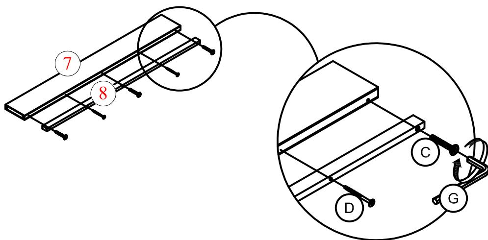
Align the Mounting Position on the Foot Cross Bar (8) to the Footboard (7). Attach the Foot Cross Bar (8) to the Footboard (7) by using 3 Bolts (C), 2 Screws (D) with Allen Wrench (G) and a Screwdriver (Not Provided).
