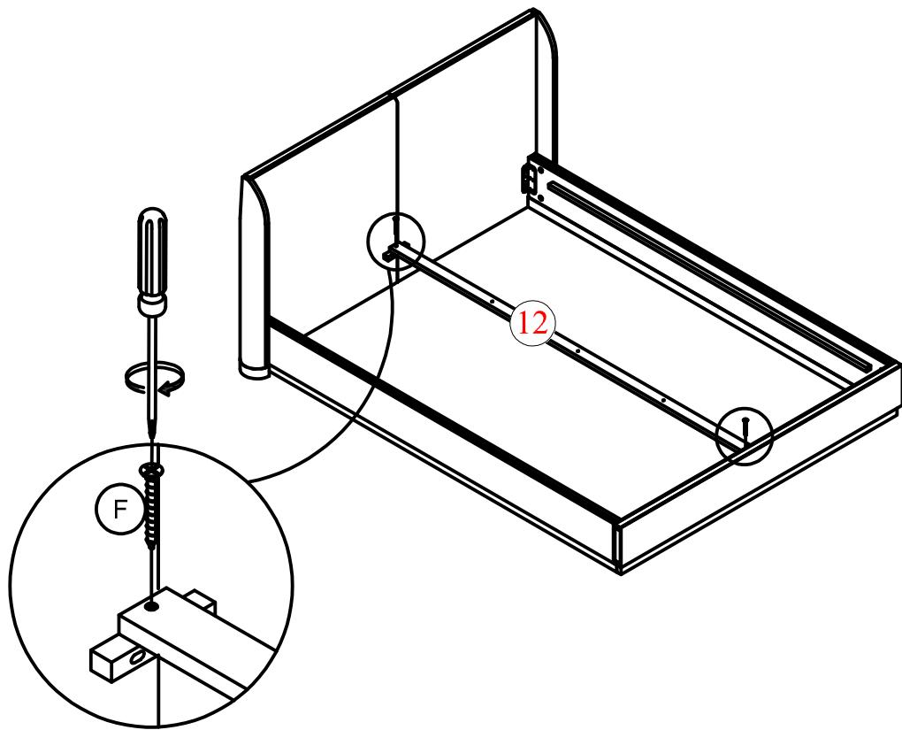
Fix the Slats Support Bar (12) to the Wooden Bar (9) by using 2 Screws (F) and a Screwdriver (Not Provided).
