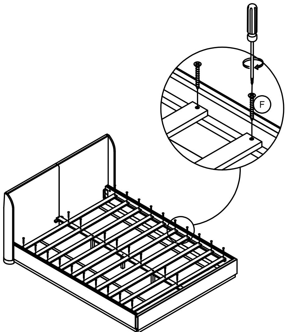
Fix the Slats (10)/(11) to the Left / Right Side Rails (5A)/(5B) and the Slats Support Bar (12) by using 28 Screws (F) and a Screwdriver (Not Provided).
