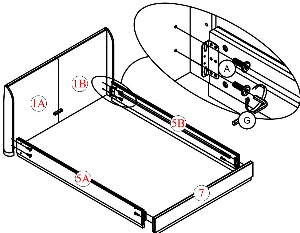
With the help of your partner, stand the completed the Footboard (5) and Headboard from Step 8 as shown in the picture above. Affix by using 8 Bolts (A) with Allen Wrench (G).
