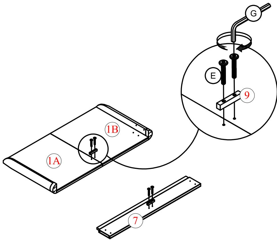
Attach the Wooden Bar (9) to the Headboard and the Footboard by using 4 Bolts (E) with Allen Wrench (G).
