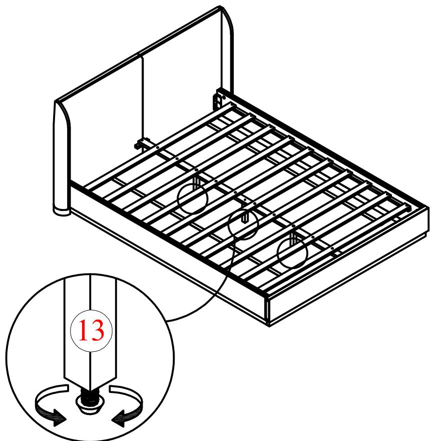
Rotate counterclockwise to increase the length of Floor Leveler, and raise that corner.
