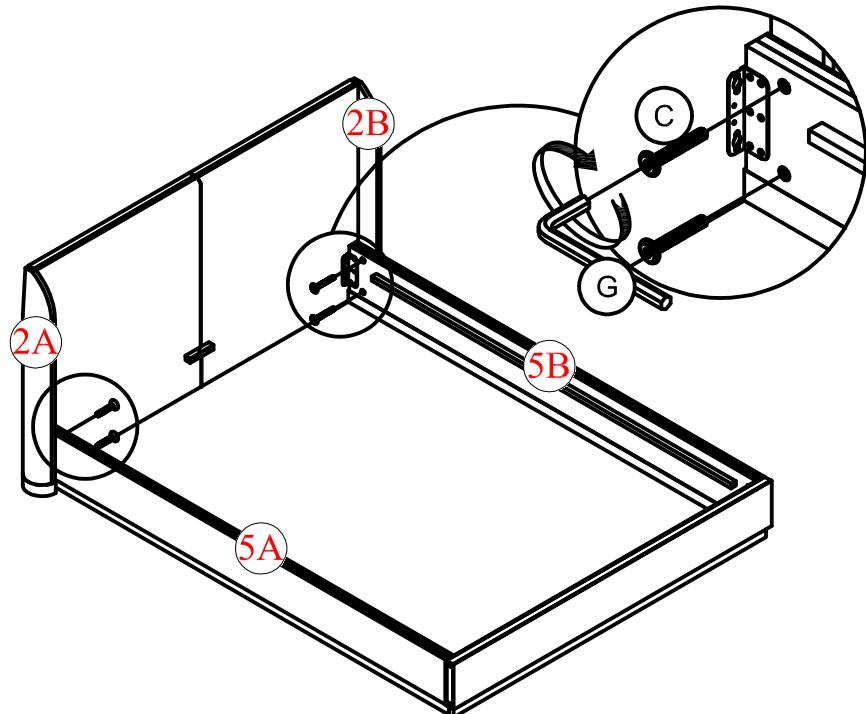
Attach the Left/Right Side Rail (5A)/(5B) to the Left/Right Headboard Side (2A)/(2B) by using using 4 Bolts (C) with Allen Wrench (G).
