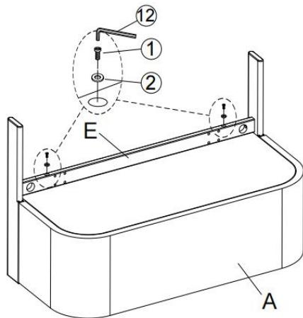
Attach Front Stretcher (E) to Seat Frame (A), by using Bolt(①), Flat Washer (②) and Allen Wrench (⑫), as pictured above.
