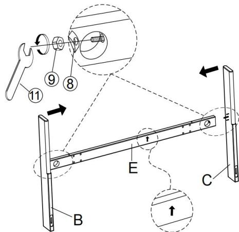
Attach Front Leg (B&C) to Front Stretcher (E), by using Half Moon Washer (8), Nut (9) and Open wrench (11), as pictured above.
