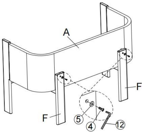
Attach Back Leg (F) to Seat Frame (A), by using Bolt(④), Flat Washer(⑤) and Allen Wrench (⑫), as pictured above.
