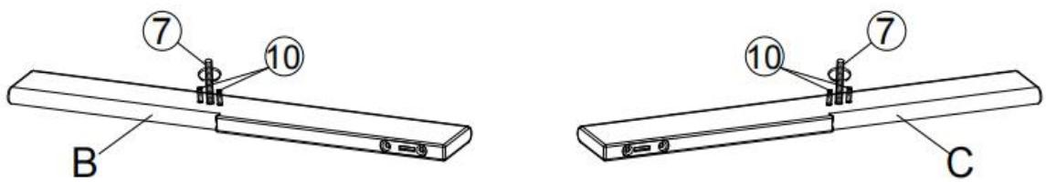
Attach Full Thread Screw (7) and Wood Dowel (10) to Front Leg (B&C), as pictured above.
