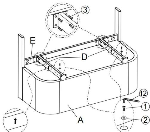
Attach Side Stretcher (D) to Front Stretcher (E), by using Bolt(③).
