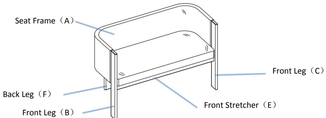
This Chair has multiple parts and may require up to some 30 minutes to assemble. To give you an overview of the Chair parts, the above picture is to help you put the various parts into perspective. Please read through the instructions below to familiarise yourself with the parts and steps before assembly.
