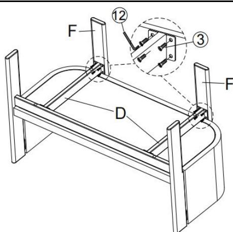
Attach Back Leg (F) to Side Stretcher (D), by using Bolt(③) and Allen Wrench (⑫), as pictured above.
