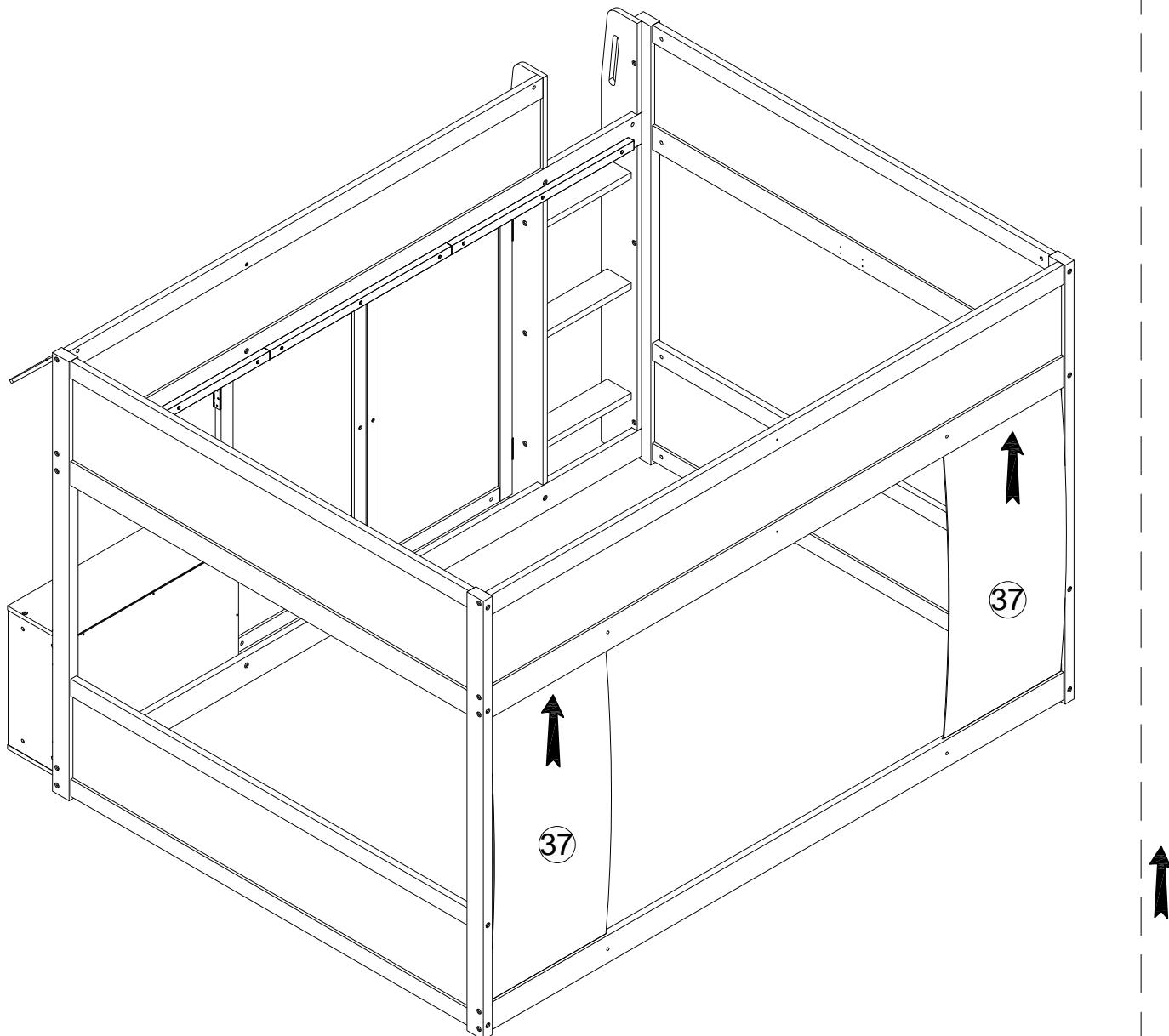
Note : Insert one end of the back panel into the bed rail groove → Bend slightly
