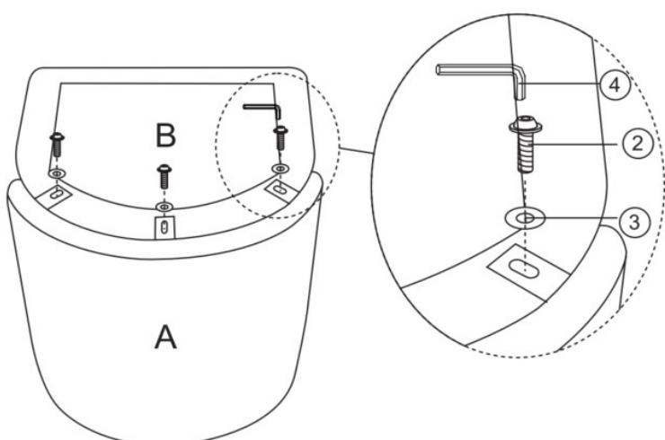
Attach the Back (A) to Seat (B) using the Washer (③) and Bolt (②) with Allen Wrench (④) as shown above.
