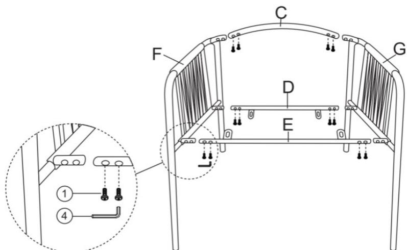
Attach the Back Connection Rod (C), Short Connection Rod (D) and Long Connection Rod (E) to Left Leg (F) and Right Leg (G) using the Bolt (①) with Allen Wrench (④) as shown above.
