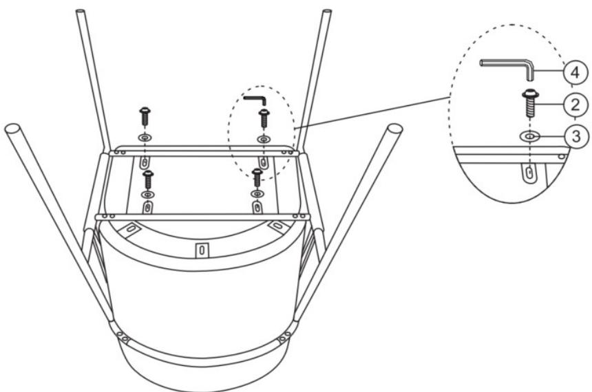
Attach the Seat (B) to the assembled left frame using the Washer (③) and Bolt (②) with Allen Wrench (④) as shown above.
