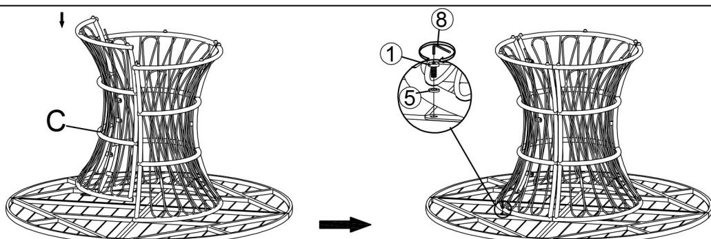
Secure the legs C to the table top with bolts (1), washers (5) and allen wrench (8)
