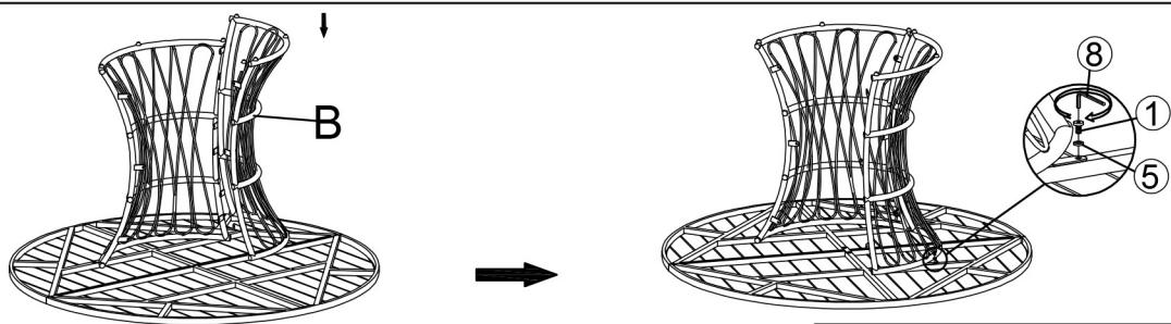
Secure the legs B to the table top with bolts (1), washers (5) and allen wrench (8)
