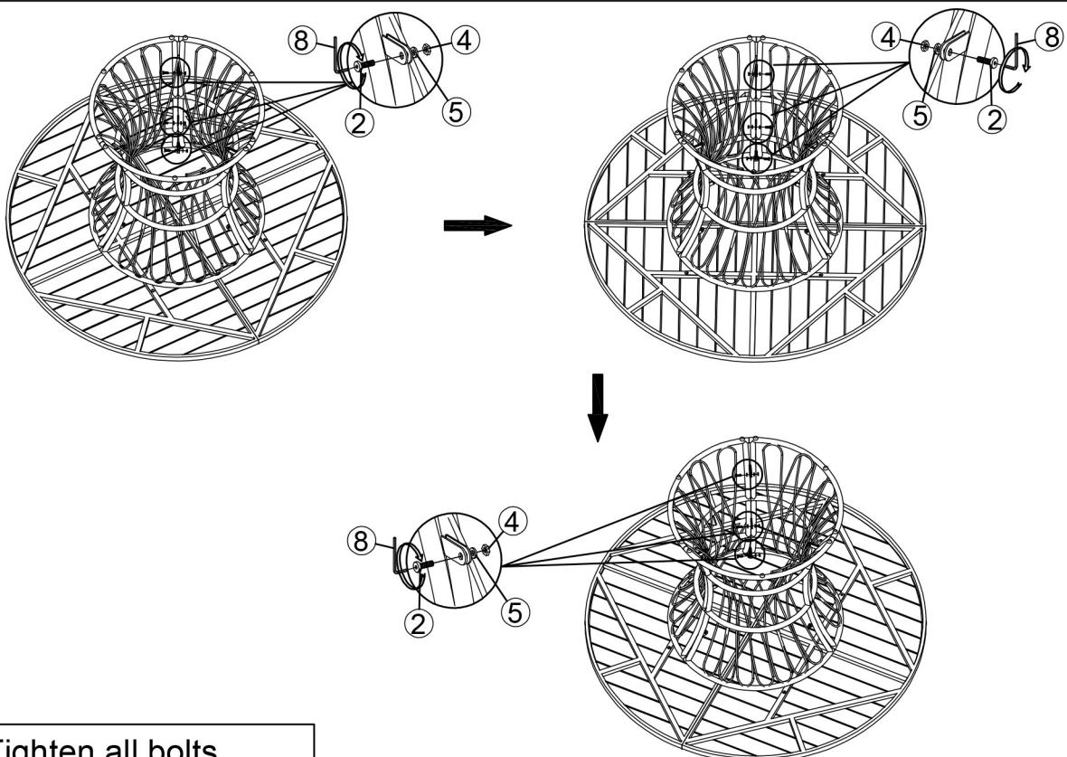
Secure legs B, C and D with bolts (2), washers (5), eru (4) and allen wrench (8)
