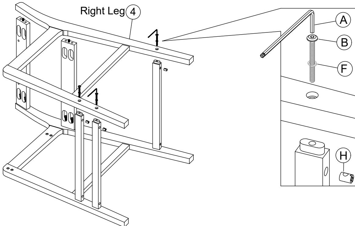
Turn the chair frame onto its side and place the Left Leg (3) flat on a soft surface. Align the mortises on the Right Leg (4) with the tenons of the Stretchers (7) and Back Rails (5 & 6), then fit them together securely. Fasten the Stretchers (7) using JCBC Bolts M6 × 60 (B), Barrel Nuts (H), and Spring Washers (F). Tighten the bolts with the Allen Wrench (A). Do not fully tighten at this stage.
