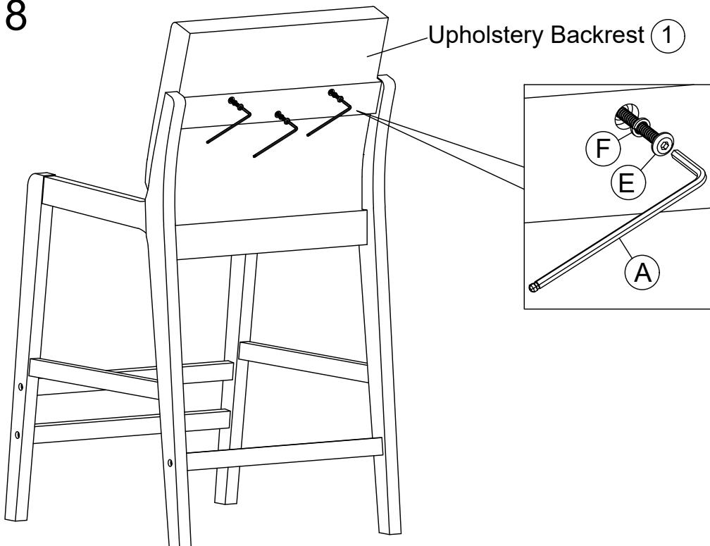
Attach the Upholstered Backrest (1) to the Upper Back Rail (5) using JCBC Bolts M6 x 35 (E) and Spring Washers (F).
