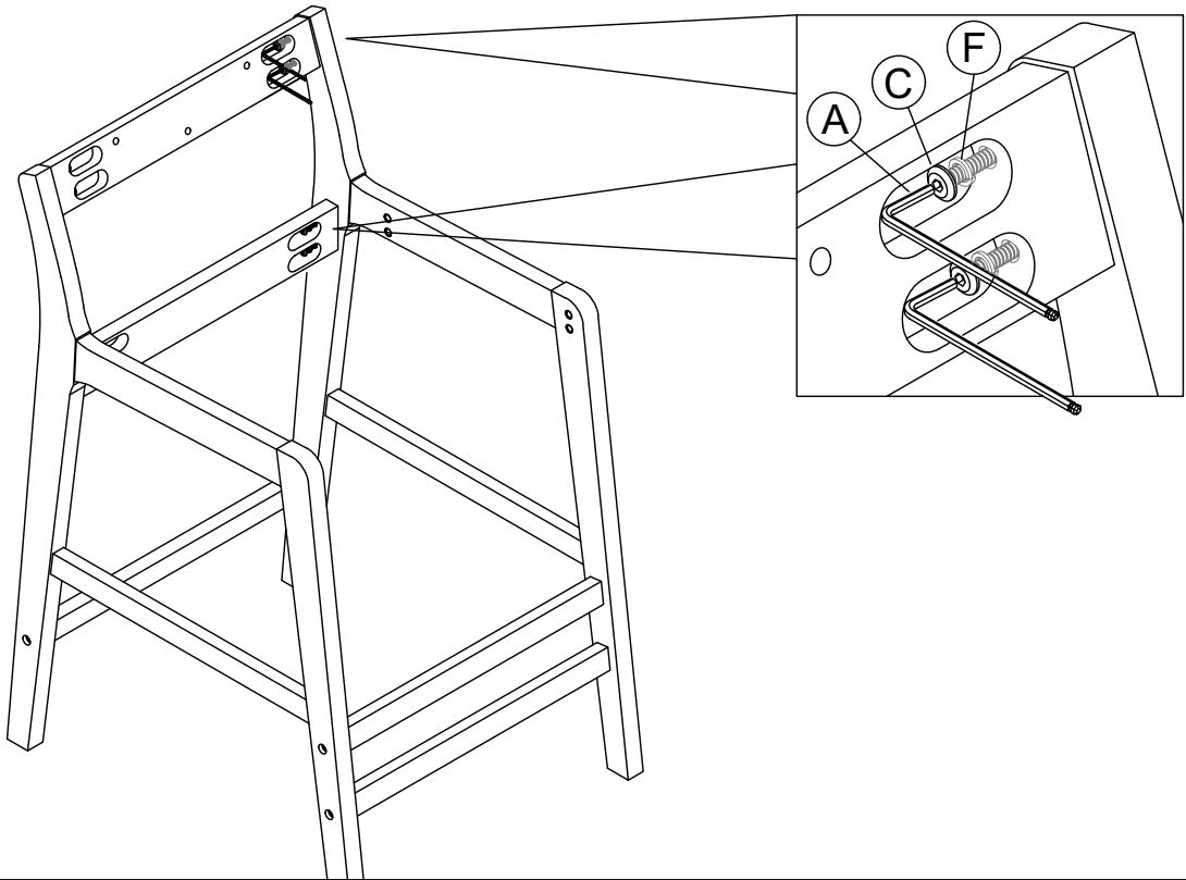
Turn the chair upright and place it on a level surface. Fasten the parts using JCBC Bolts M6 × 50 (C) and Spring Washers (F). Tighten the bolts with the Allen Wrench (A). Do not fully tighten at this stage.
