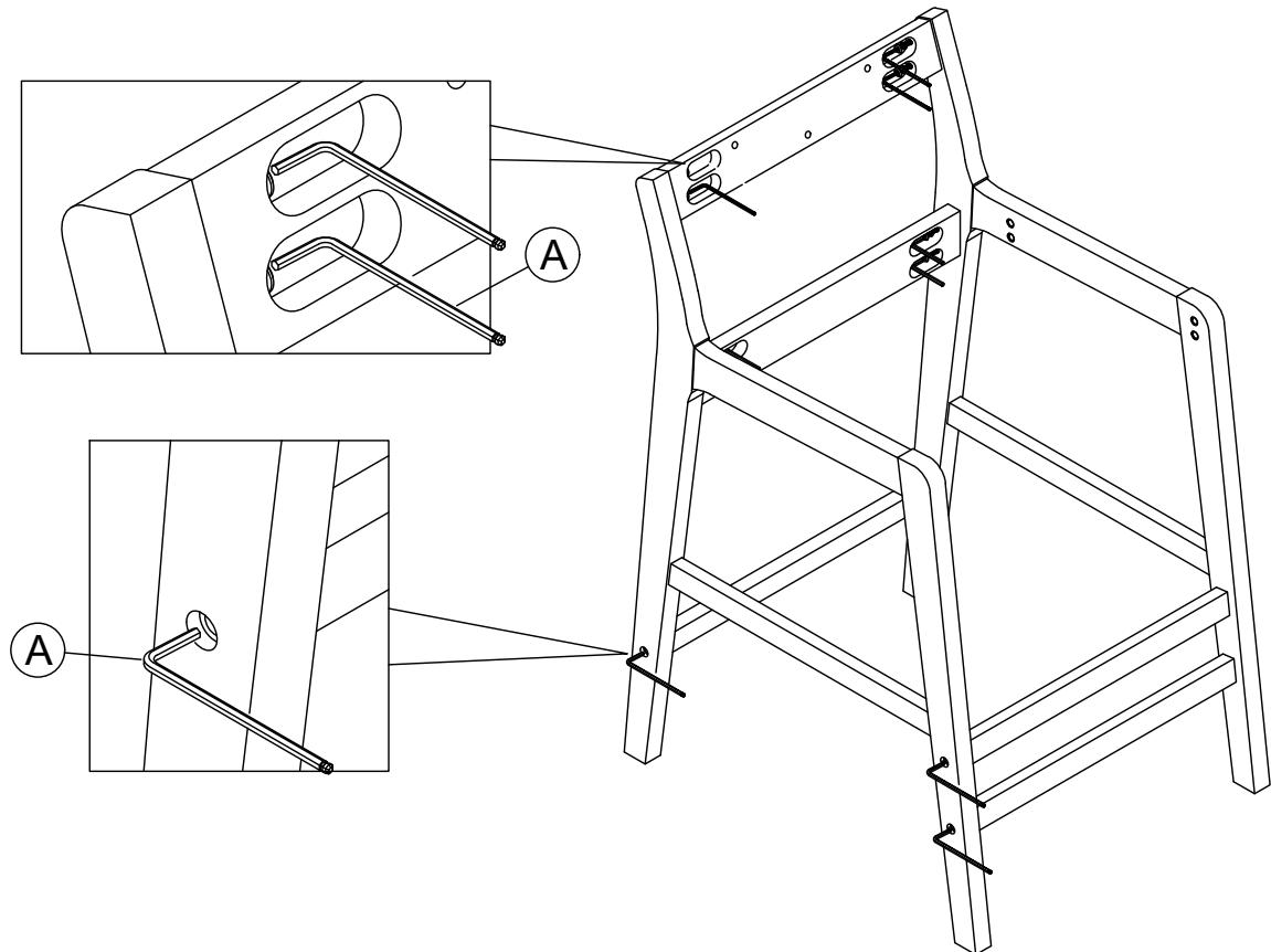
Make sure all four legs rest evenly on the floor, then use the Allen Wrench (A) to fully tighten all previously loosened bolts.
