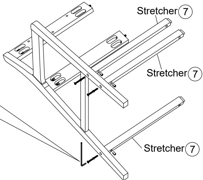
Attach the three Stretcher (7) to the Left Leg (3) using JCBC Bolts M6 x 60 (B), and Spring Washers (F) and Barrel Nut (H) .
