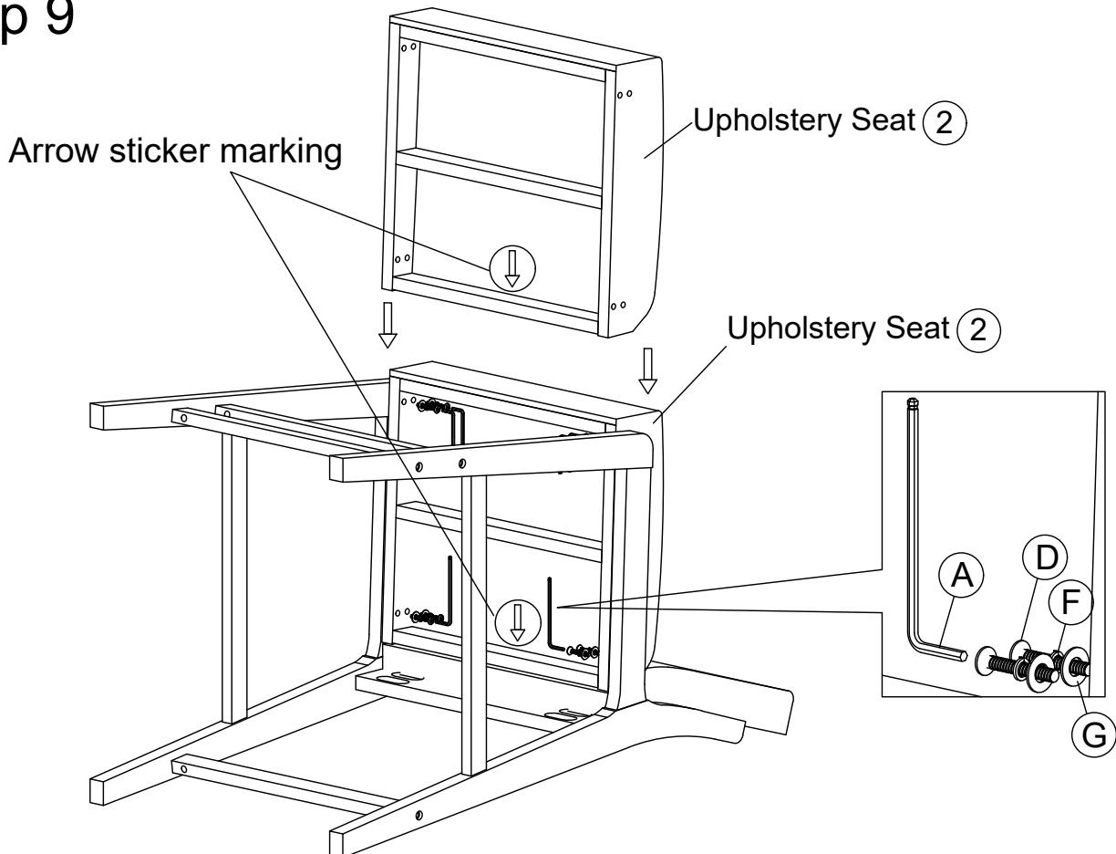
Turn the Bar stool so that the backrest faces down, and place it on a soft surface. Attach the Upholstered Seat (2) to the Left Leg (3) and Right Leg (4) using JCBC Bolts M6 × 40 (D), Spring Washers (F) and Flat Washer (G). Insert all eight bolts by hand and tighten them slightly, then secure them firmly with the Allen Wrench (A).
