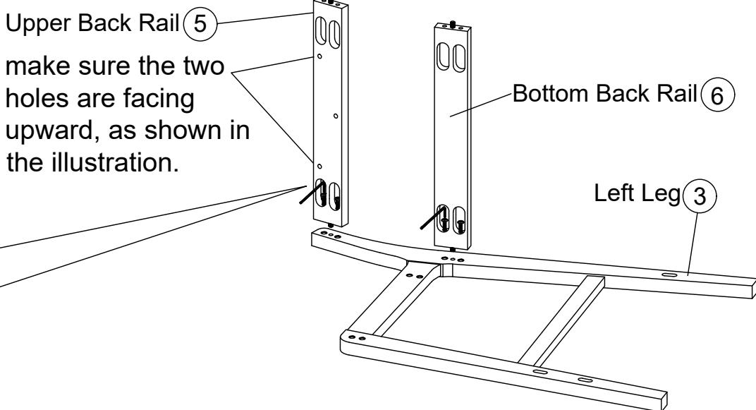
Attach the Upper Back Rail (5) and Bottom Back Rail (6) to the Left Leg (3) using JCBC Bolts M6 x 50 (C) and Spring Washers (F).
