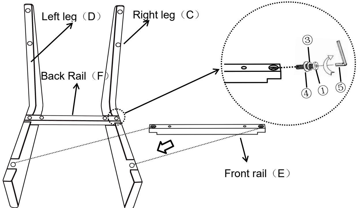
Attach the Rails(E+F) into the mounting positions of the Legs(C+D) using Bolts(①), Spring Washer(③) and Washer(④) with Allen Wrench(⑤).
