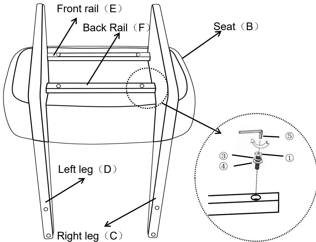
Place the assembled frame on the Seat (B) with the bottom facing you, as shown in the picture above.
