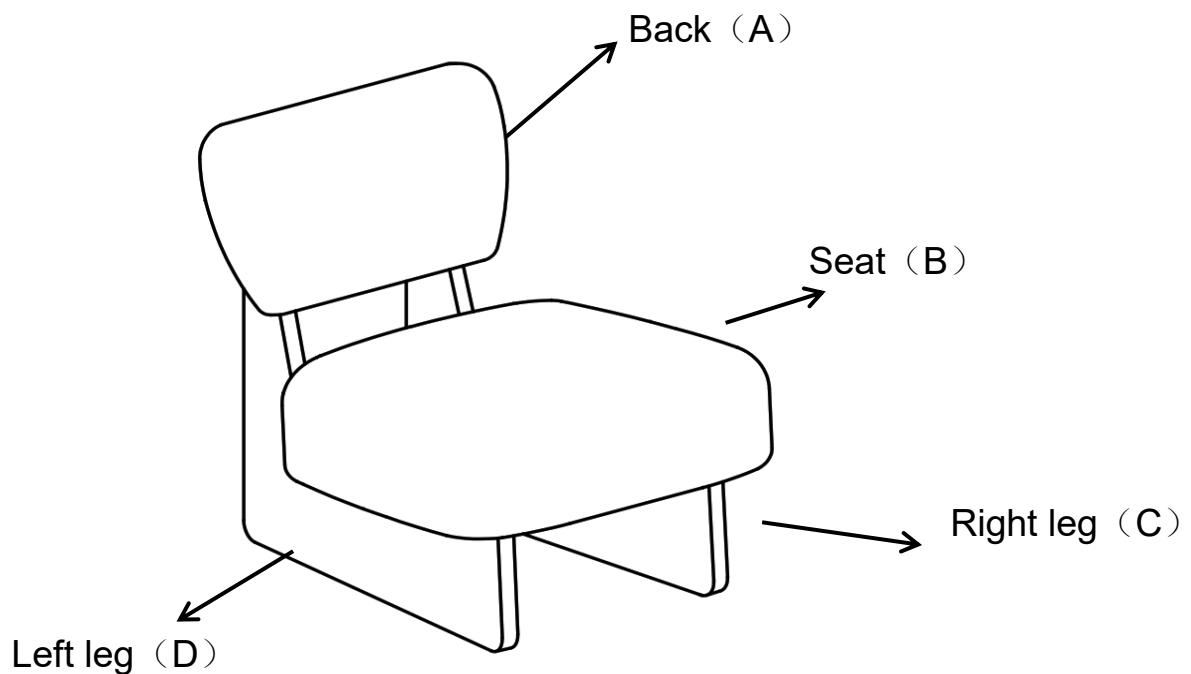
Check for stability and then tighten all the remaining bolts. DO NOT fully tighten a bolt in one go and then move on to the next. Rather, in a sequential manner, gradually tighten each bolt until all bolts are evenly secured. This methodology will ensure maximum evenness once all bolts are fully tightened.
