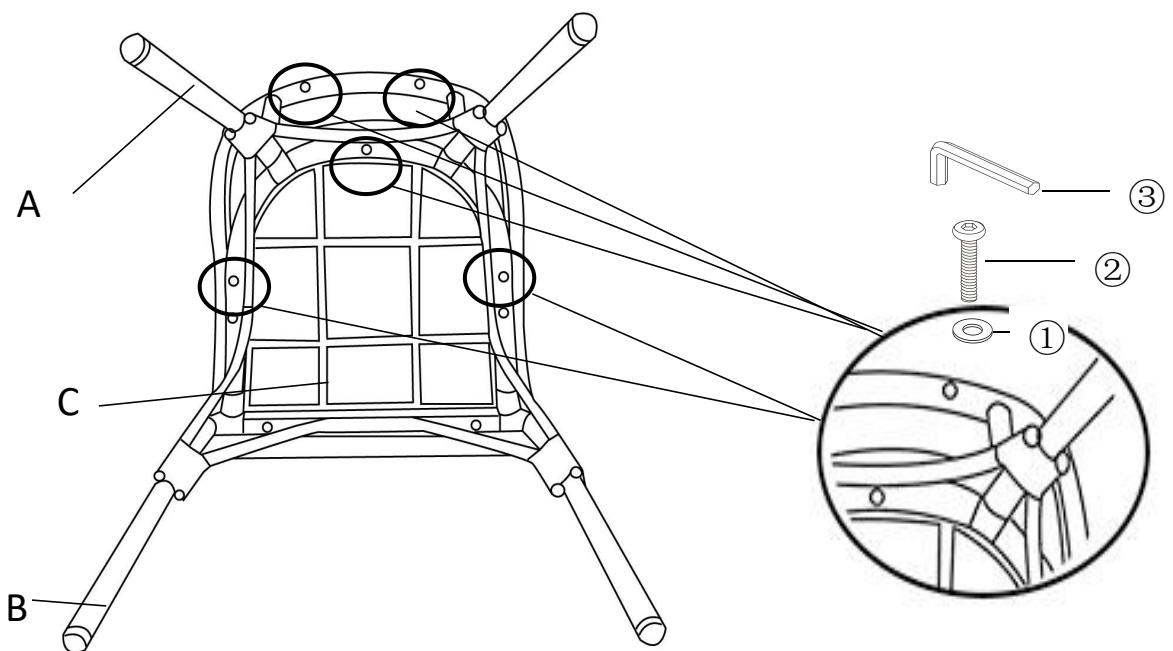
Attach the Seat(C) to the Backseat(A) with Washers(①) and Bolts(②) using the Allen Wrench(③) as shown above.
