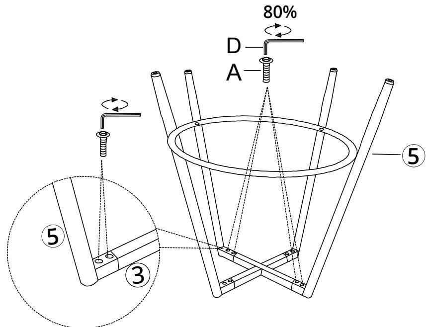
Remark: Please install the remaining two legs and tighten the Bolts A to around 80%.
