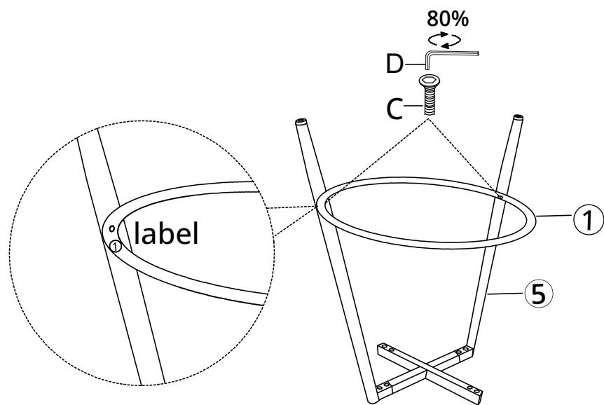
Remark: Please secure the Footrest to both legs and tighten the Bolts C to around 80%.
