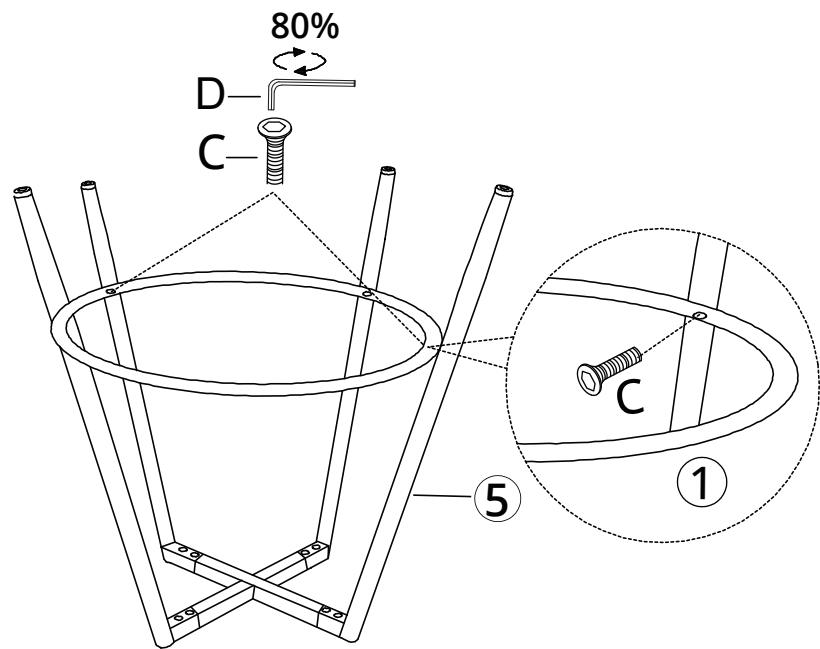
Remark: Please secure the Footrest to the other two legs and tighten the Bolts C to around 80%.
