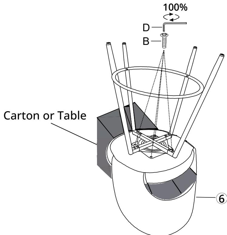
Remark: Tighten the four Bolts B connecting the Seat to 100%.
