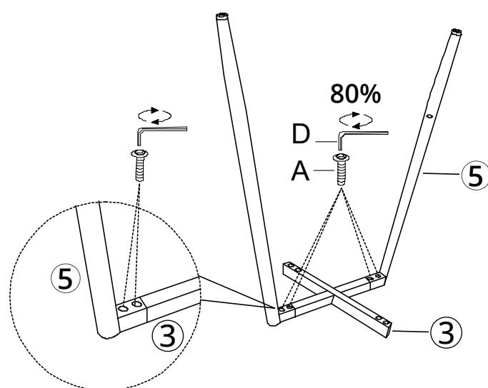
Remark: Please install the two legs first and tighten the Bolts A to around 80%.
