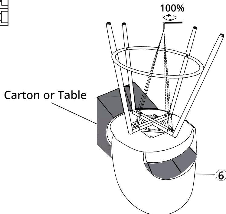
Remark: Tighten the connecting Bolts between the four legs to 100%
