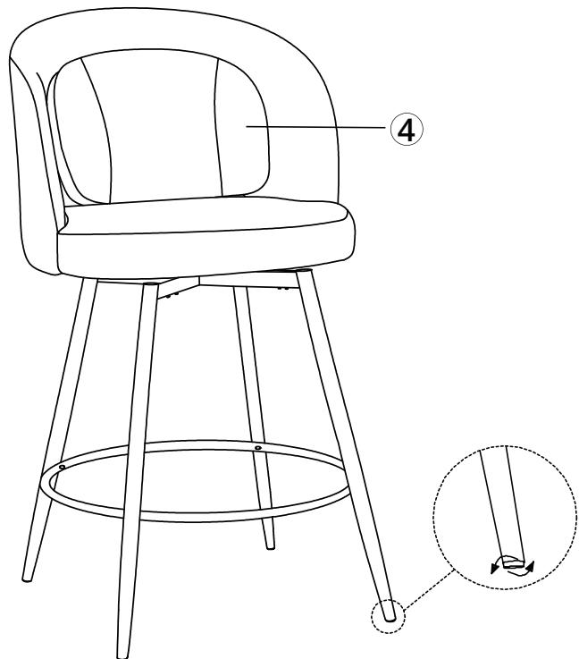
Remark: Adjust leveling feet for balance.
