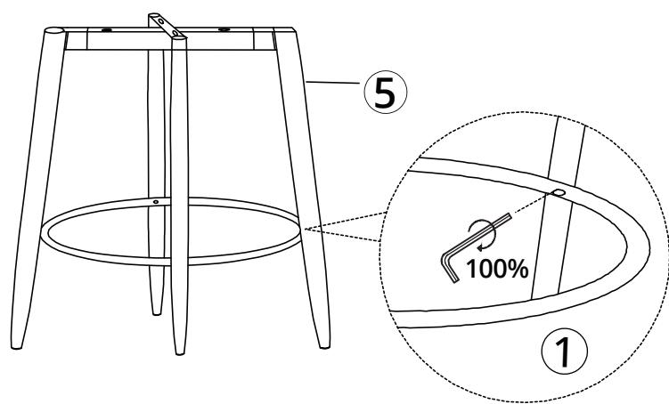
Remark: Place the bar stool base flat, then completely tighten all Bolts on the Footrest to 100%.
