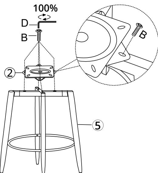
Remark: Rotate the Swivel Plate to make the upper and bottom parts cross and separate. Then tighten the four Bolts B connecting the legs to 100%.
