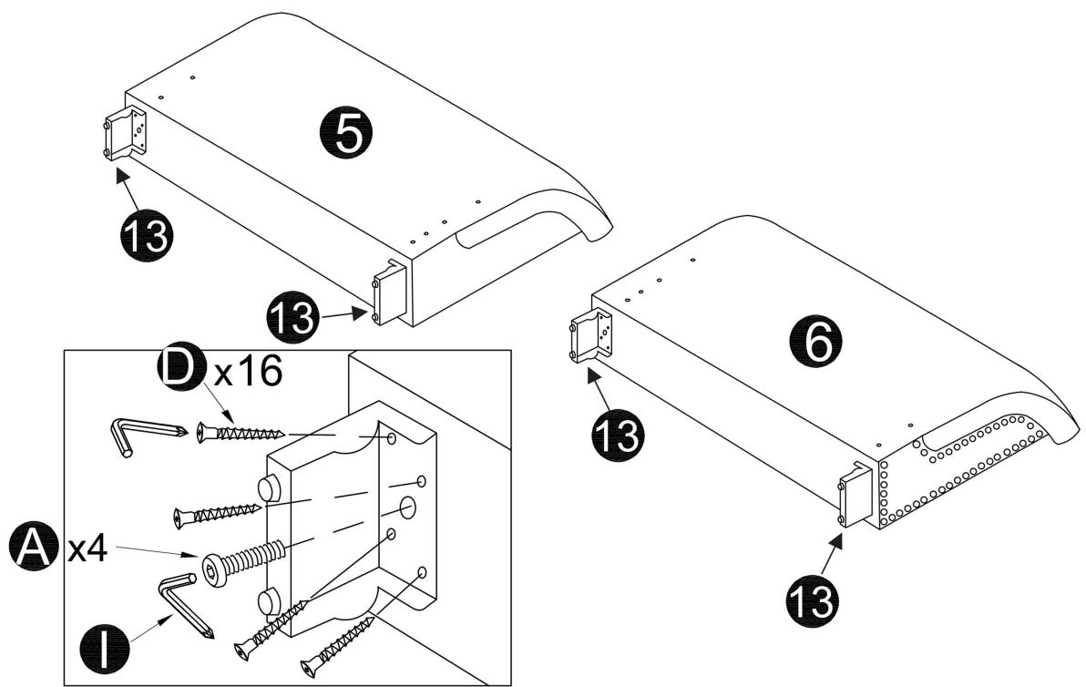
**Fix No. 13 onto No. 5 and No. 6 with hardware E**
