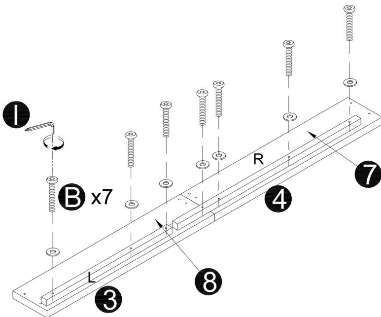
Use hardware B to pass through hardware C and fix numbers 7 and 8 onto numbers 3 and 4
