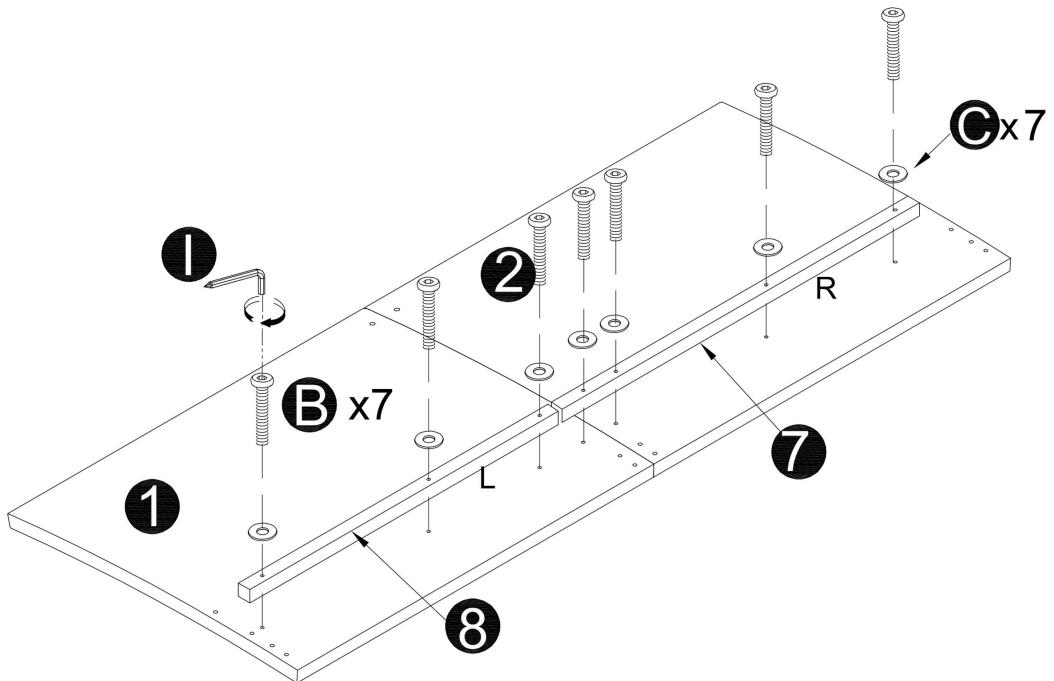
Use hardware B to pass through hardware C and fix numbers 7 and 8 onto numbers 1 and 2
