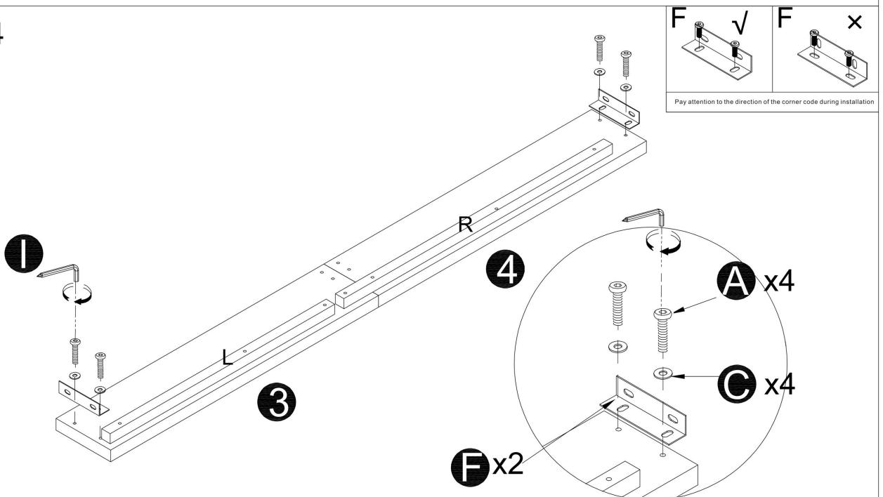
Use hardware A to pass through hardware D and C, and fix hardware F on numbers 3 and 4 (as long as the screw is locked to 80%)
