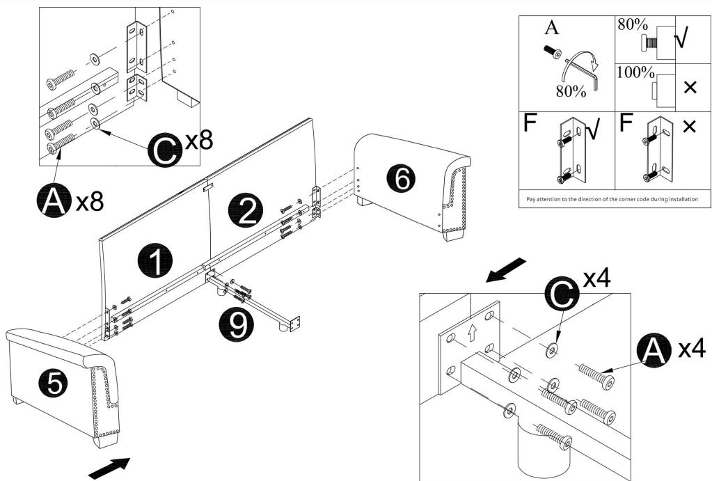
Connect the components of the front group together by threading hardware A through hardware D and C according to the diagram. All screws only need to be locked to 80%
