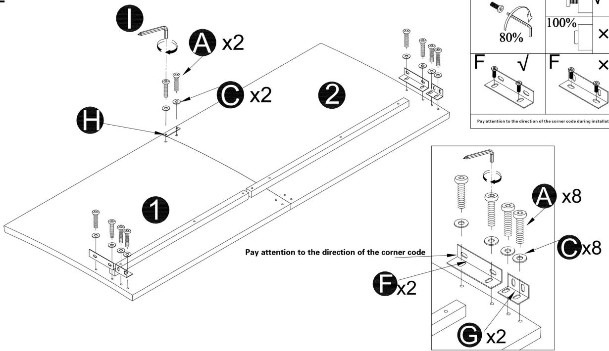
Use hardware A to pass through hardware D and C, and fix hardware I&F&G on screws 1 and 2 as long as they lock to 80%
