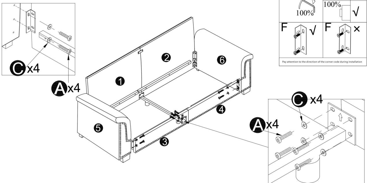
Connect the components of the front group together by threading hardware A through hardware D and C according to the diagram. All screws only need to be locked to 100%
