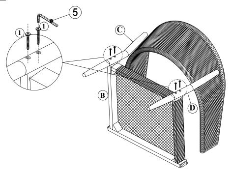
Align the Seat Chair (B) with the two Back Legs (D) and (C), matching the holes as illustrated. Attach the two Seat Chair (B) and with the two Back Legs (D) and (C), using Screws (1) and Allen Wrench (5) as shown in the illustration.
