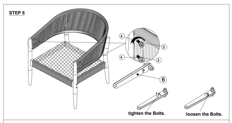
Attach the two Back Frame (A), and with the two Front Legs (F) and (E), using bolts (3), washer (4) and Ratchet Tool(6) as shown in the illustration.
