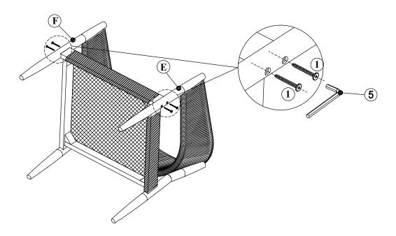
Align the Back Frame (A), Seat Chair (B) with the two Front Legs (F) and (E), matching the holes as illustrated. Attach the two Back Frame (A), Seat Chair (B) and with the two Front Legs (F) and (E), using Screws (1) and Allen Wrench (5) as shown in the illustration.
