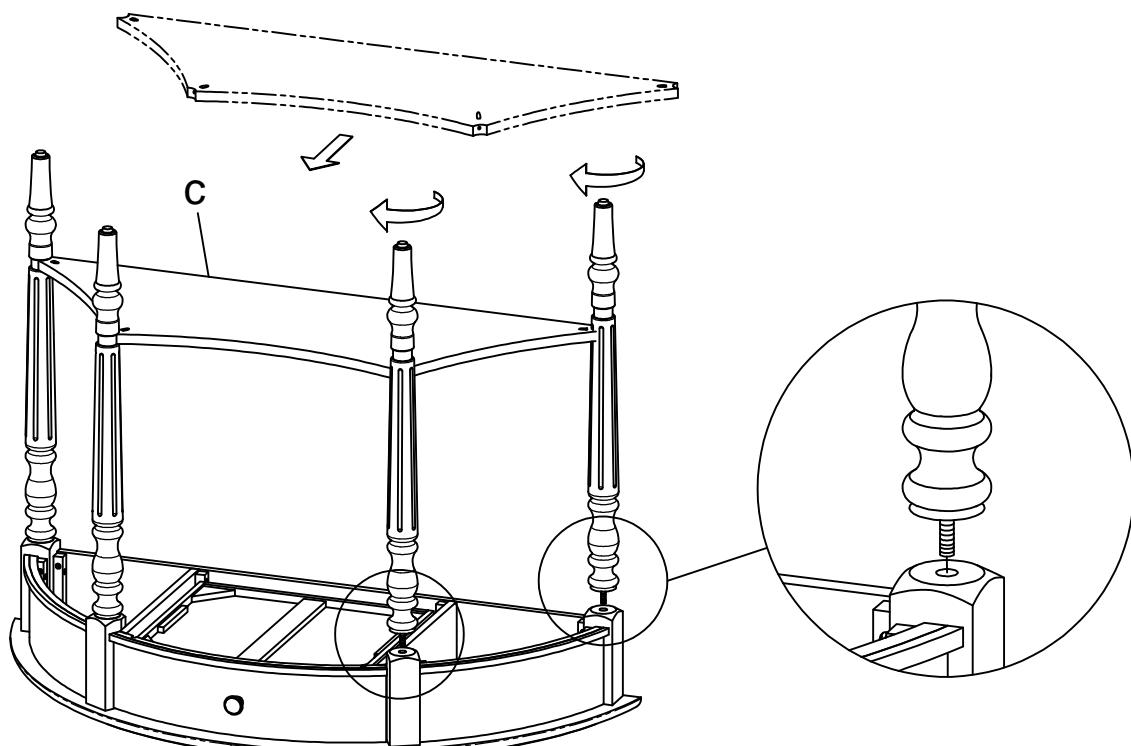
After tightening the 4 table legs (B) use wood screws (1) to fix the 4 drilled holes on the table base in the correct position.
