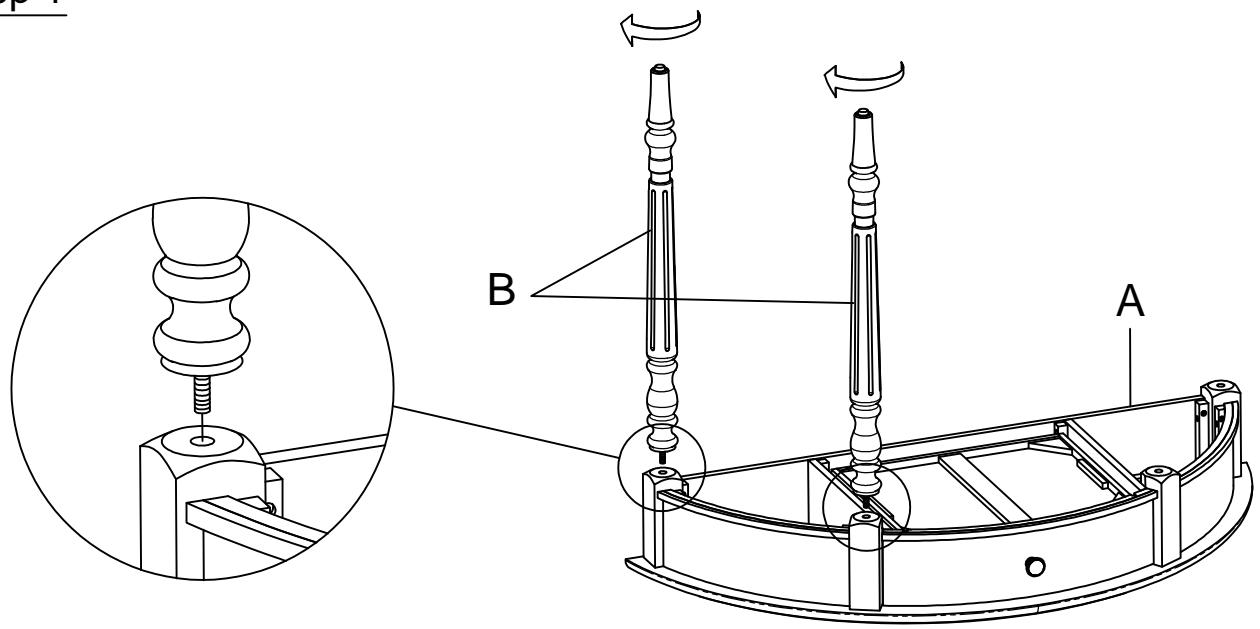
Need someone to help put the table shelf into the correct recess on the table leg, assemble the 2 right legs and tighten them.
