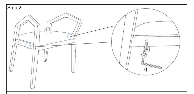
Use Bolts(1) with Allen Wrench(4) to tighten it.
