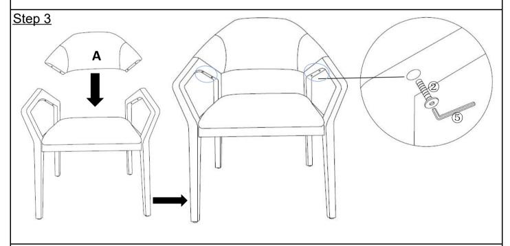
Take out Backrest(A), insert it downwards to make the holes of Backrest and leg aligned as shown. Use Bolts(②) with Allen Wrench(⑤) to tighten it.
