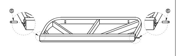
Install the Wooden Tenons(©) into the sides of the Seat cushion(F) as pictured above.
