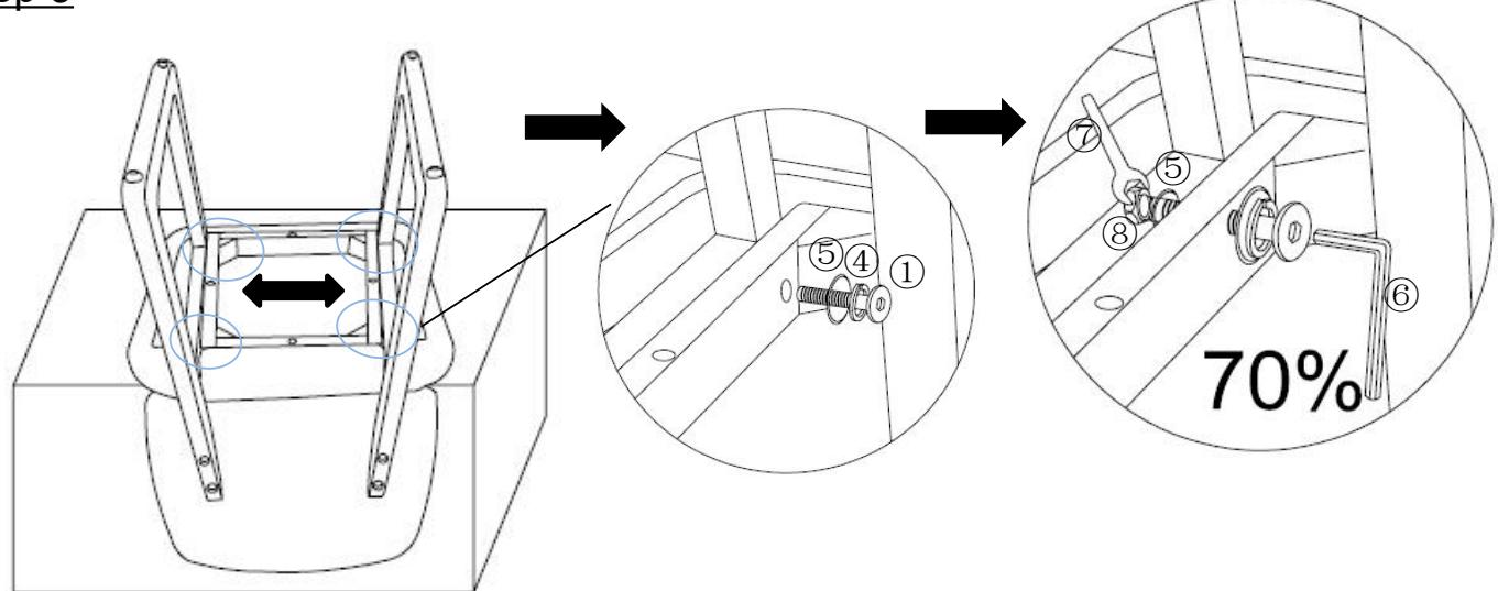
Use Bolts(①) Spring Washer(④),Flat Washer(⑤), insert it from the inner side hole of the Seat Frame(C) into the outside, then put the Flat Washer(⑤), Nut(⑧) onto Bolts(①) from the outside, and lock with Wrench(⑦). Then lock the Bolts(①) with Allen Wrench(⑥) .
