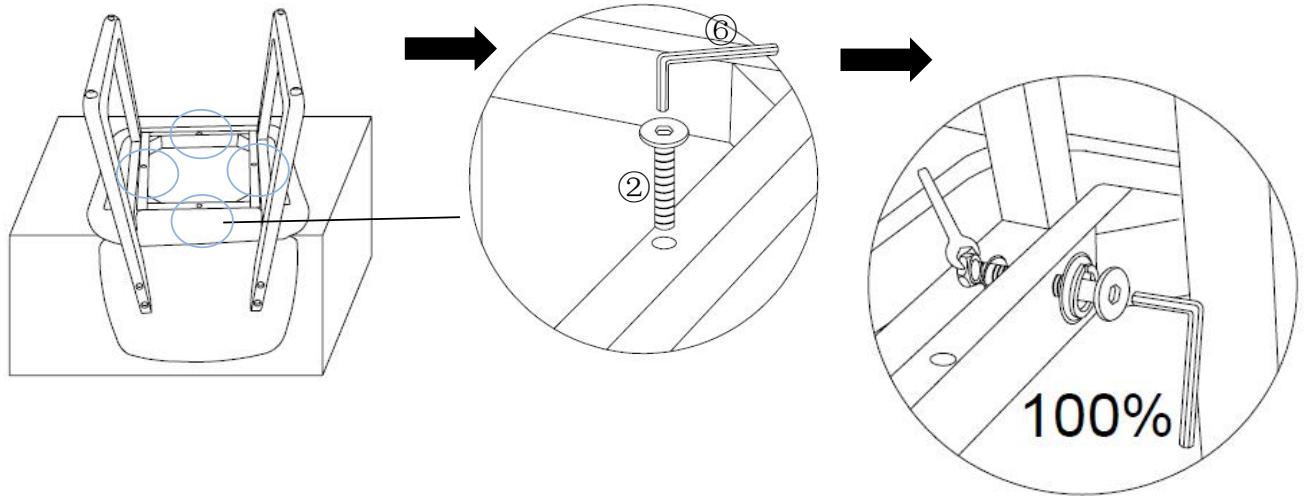
Insert Bolt(②) into the holes of the Frame(C) with Allen Wrench(⑥) to lock it
