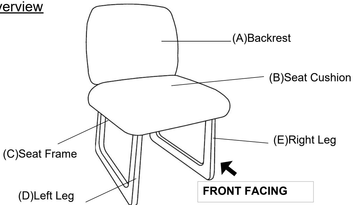
This Chair has multiple parts and may require up to 30 minutes to assemble. To give you an overview of the Chair parts, the above picture is provided to help you put the various parts into perspective. Please read through the instructions below to familiarise yourself with the parts and steps before assembly.
