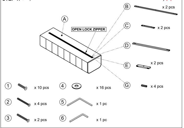
STEP 2: Attach two the Long Rail (B) to Seat Frame Body (A) using BOLT (1), FLAT WASHER (4), and tighten them using the ALLEN KEY (5).
