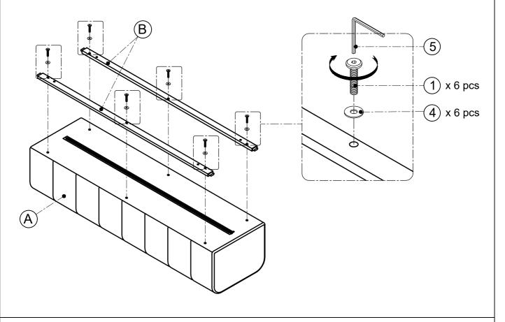
STEP 3: Attach two the Short Rail (C) to Seat Frame Body (A) using BOLT (1), FLAT WASHER (4), and tighten them using the ALLEN KEY (5).
