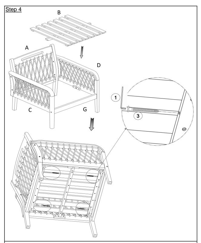
With assistance from you adult partner, attach Seat Panel (B) to the assembled part in Step 3 and then secure Seat Panel (B) to Leg Panels (C, D) by using Screws (3) with Allen Wrench (1) as shown above. **DO NOT fully tighten the Screws.**
