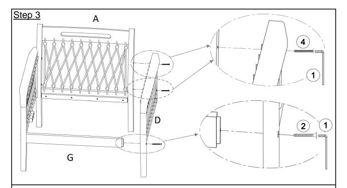
With assistance from you adult partner, attach Right Leg Panel (D) to both Front Bar (G) and Backrest Panel (A) of the assembled part in Step 2 then secure by using Screw ((2)), Bolts ((4)) with Allen Wrench ((1)) as shown above.
