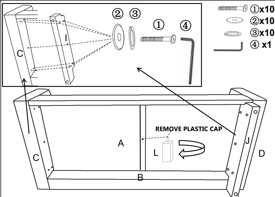
**Place the assembled parts horizontally and use screws (①) to install the leg(I)(J). flat washer (②), as well as spring washer (③).tighten screws (①) with allen wrench (④ ).remove paastic cap,rotate the central leg (L) into the hole at the bottom of the sofa.**
