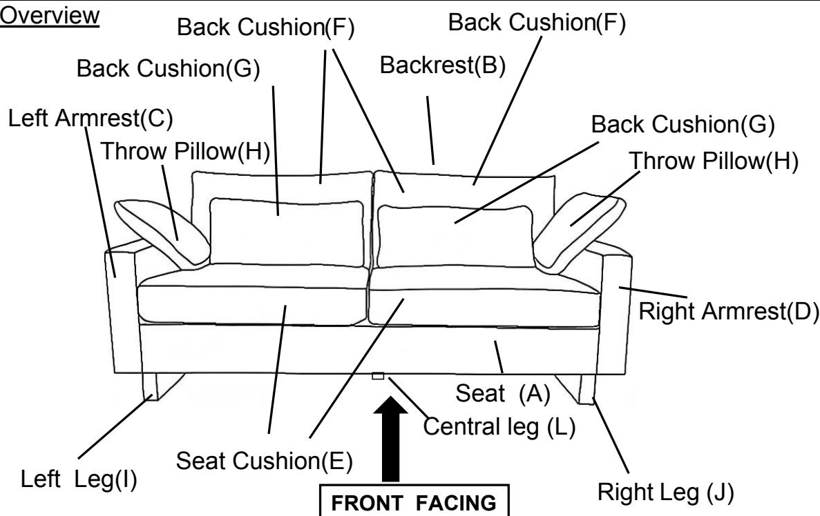
This sofa has multiple parts and may require up to some 30 minutes to assemble. To give you an overview of the sofa parts, the above picture is to help you put the various parts into perspective. Please read through the instructions below to familiarise yourself with the parts and steps before assembly.
