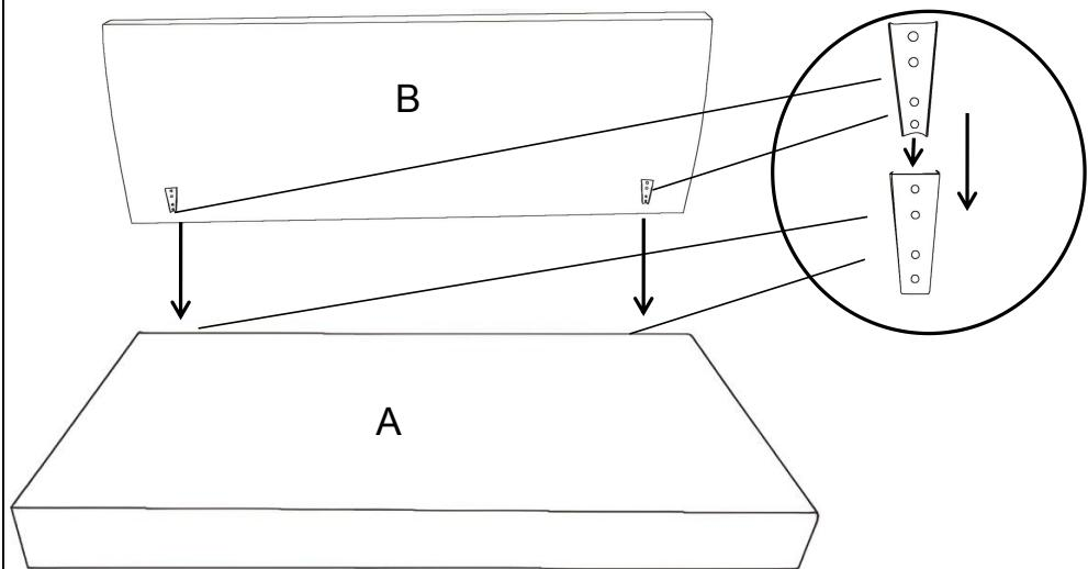
**Place the sofa seat (A) vertically and connect the pin on the backrest (B) and the pin on the sofa seat (A) together.**
