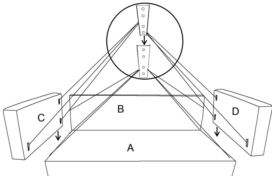
**Place the assembled sofa seat (A) and backrest (B) vertically, and connect the dowels on the armrests (C) (D) the dowels on the sofa seat (A) and backrest (B).**
