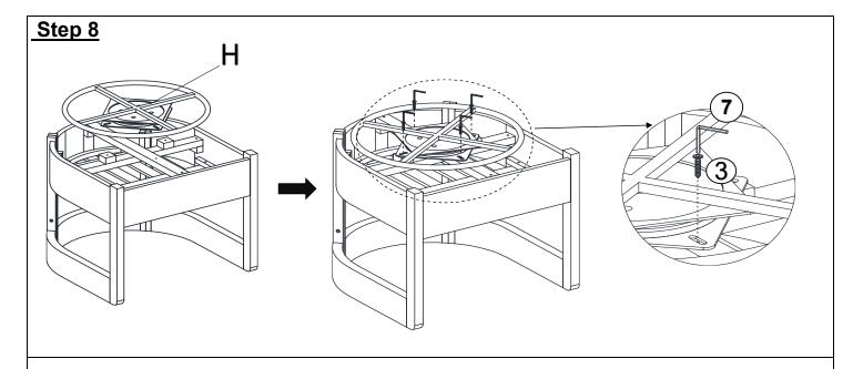
Attach the Swivel Base (H) to the assembled part in Step 7 by using Screws (③) and the Allen Wrench (⑦). **Do not fully tighten the Screws at this time**
