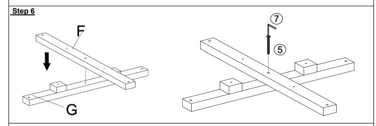
Place the Support Swivel 2 (G) and the Support Swivel 1 (F) as shown in picture above. Attach the Support Swivel 1 (F) to the Support Swivel 2 (G) by using Screws (5) and the Allen Wrench (7). **Do not fully tighten the Screws at this time**
