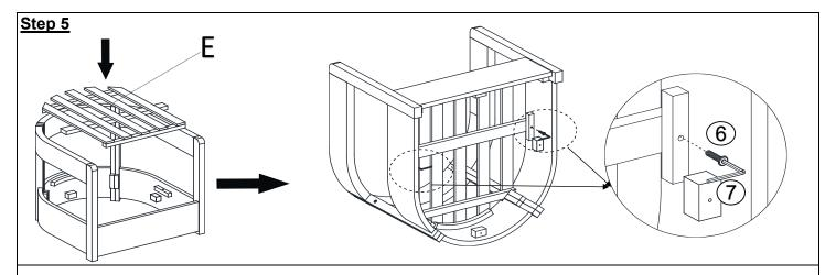
Place the Seat Panel (E) and the assembled part in Step 4 as shown in picture above. Attach the Seat Panel (E) to the assembled part in Step 4 by using Screws (⑥) and the Allen Wrench (⑦). Note: Insert the Screws (③) from the inside to the outside of the Seat Panel (E)
