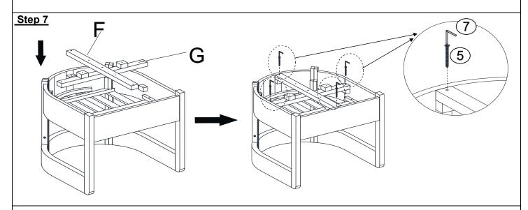
Upside down the assembled part in Step 5 and attach assembled part in Step 6 to the assembled part in Step 5 by using Screws (⑤) and the Allen Wrench (⑦).
