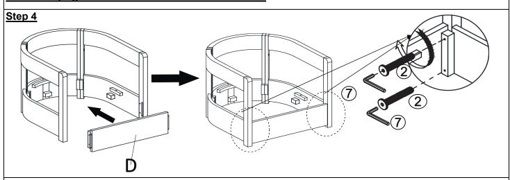
Attach the Support Bar (D) to the assembled part in step 3 by using Bolts (2) and the Allen Wrench (7) as shown above.
