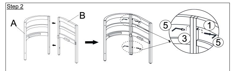
Place the Backrest Panel (A) upright as shown in the picture above onto a clean, soft surface to avoid any scratches or damages to the product.
