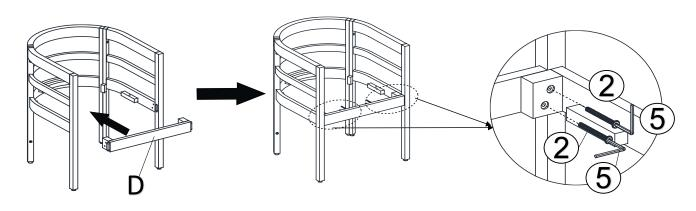
Attach the Support Bar (D) to the assembled part in step 3 by using Bolts (2) and the Allen Wrench (5) as shown above.
