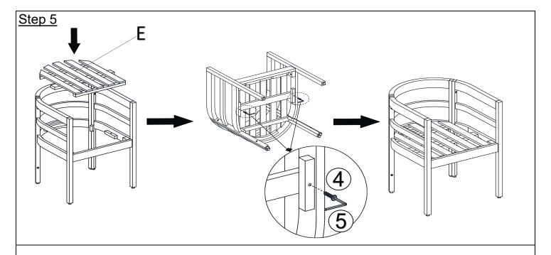
Attach the Seat Panel (E) into the Chair as shown in picture above.
