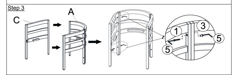
Attach the Left Leg Panel (C) to the assembled part in step 2 by using Bolts (1), Sleeve Nuts (3) and the Allen Wrench (5) as shown above.
