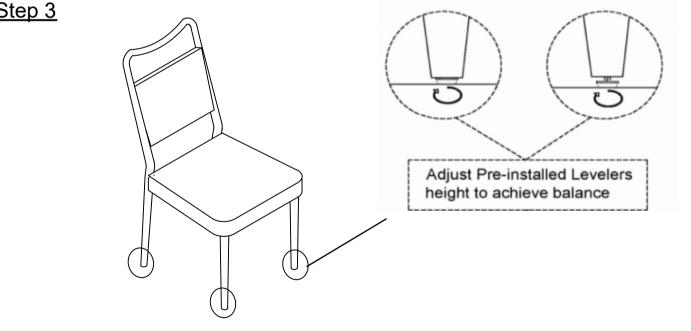
Adjust the Pre-installed Levelers at the bottom of the Legs (C) and Back With Legs (B) until the Dining Chair is level with the ground.
