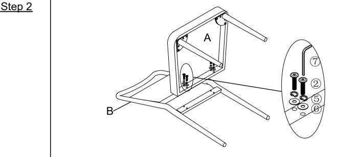
Attach the Seat( A ) to the Back With Legs( B ) with the Bolts(2) and Spring Washers (⑤) and Washers (⑥), and Allen Wrench (⑦) as shown in the figure above.
