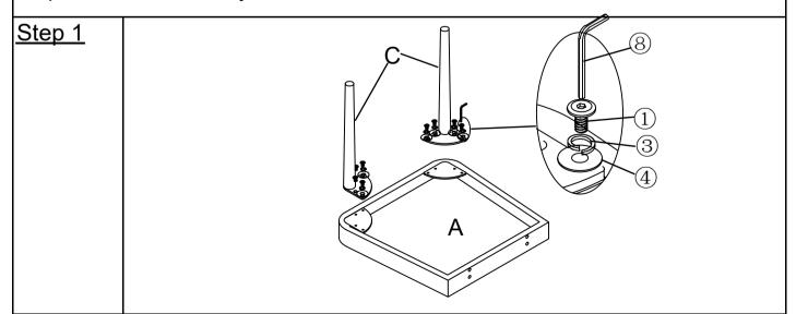
Attach the Legs (C) to the Seat (A) with the Bolts (1) and Spring Washers (③) and Washers (④), and Allen Wrench (⑧) as shown in the figure above.
