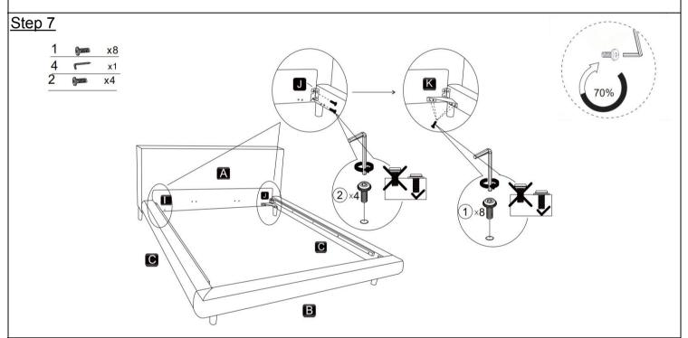
Use bolts (1) to install the two bed side plates (C) onto the headboard (A), and also use bolts (1) to install the headboard, footboard and side reinforcement hardware (K) at the connection points of the bedside and footboard W tail. Fix the two bed feet (D) onto the headboard foot hanging plate (L), and tighten them with an Allen wrench (4). Note: Do not tighten the bolt completely
