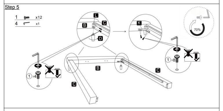
Use bolts (1) to install the two bed side plates (C) onto the bed tail plate (B), and also use bolts (1) to install the bed head, bed tail and bed side reinforcement hardware (K) at the connection points of the bed side and bed tail. Fix the two bed feet (D) onto the bed tail foot hanging plate (L), and tighten them with an Allen wrench (4). Note: Do not tighten the bolt completely.
