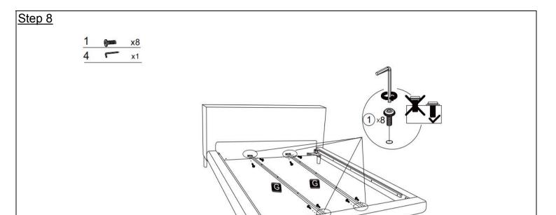
Install the headboard and footboard connecting rod (G) to the middle position between the headboard and footboard with a
