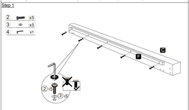
Install the rib support strip (F) on the bed side plate to the bed side plate (C) with bolts (2) and washers (3), and tighten it with an Allen wrench (4). Note: tighten the bolt completely.
