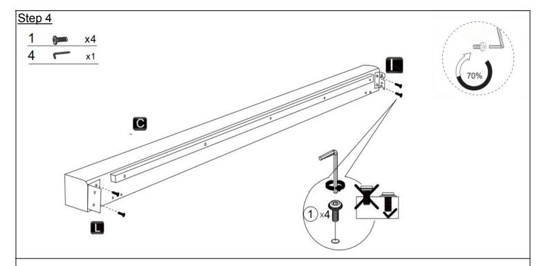
Use bolts (1) to install the left bed side and headboard connection plate (J) and the bed tail foot hanging plate (L) onto both ends of the bed side plate (C), and then tighten them with an Allen wrench (4). Note: Do not tighten the bolt completely.
