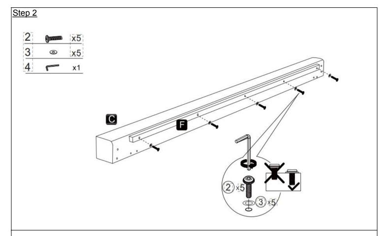
Install the rib support strip (F) on the bed side plate to the bed side plate (C) with bolts (2) and washers (3), and tighten it with an Allen wrench (4). Note: tighten the bolt completely.
