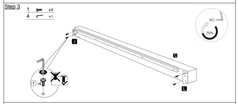
Use bolts (1) to install the left bed side and headboard connection plate (J) and the bed tail foot hanging plate (L) onto both ends of the bed side plate (C), and then tighten them with an Allen wrench (4). Note: Do not tighten the bolt completely.
