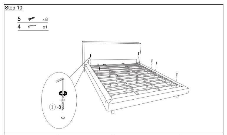
Install the bed board strip (E) onto the rib support strip (F) on the bed side panel with screws (5), and tighten it with an Allen wrench (4)
