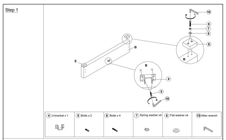
Fix the bed legs (E) to the headboard below (B) using bolts (6), spring washers (7) and Flat washers (8) by using allen wrench (10).
