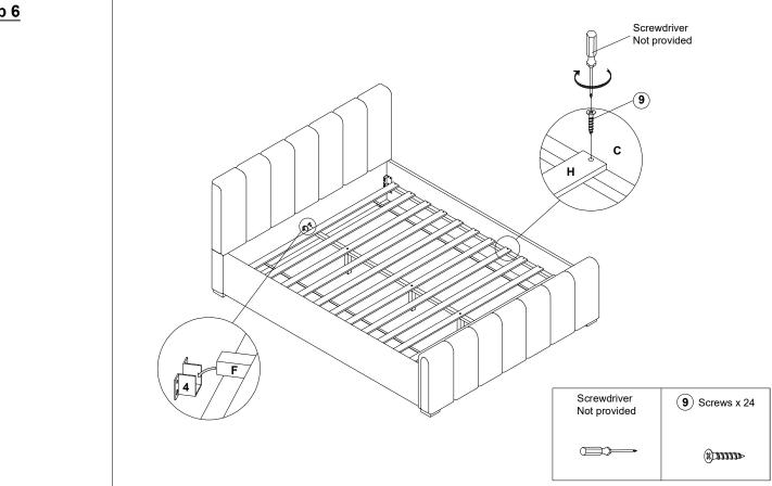
Fix the slats completed (H/F/G) the side rail (C) using screws (9), by screwdriver (Not provided) Secure the middle support bar (F) to the U-bracket (4)
