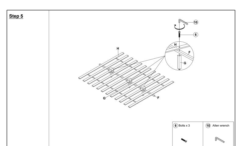
Fix the middle support legs (G) to middle support bar (F) and the slats (H) using bolts (6), by using allen wrench (10).
