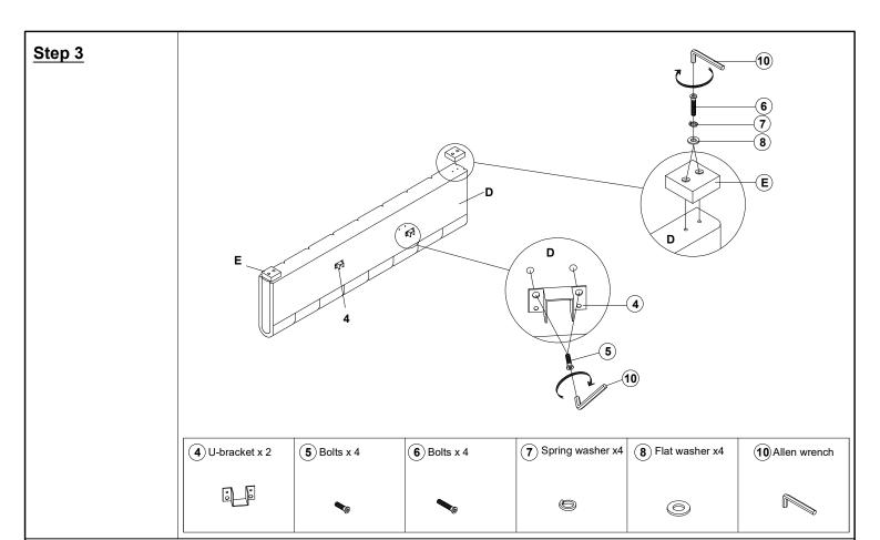
Fix the bed legs (E) to the footboard (D) using bolts (6), spring washers (7) and Flat washers (8) by using allen wrench (10).
