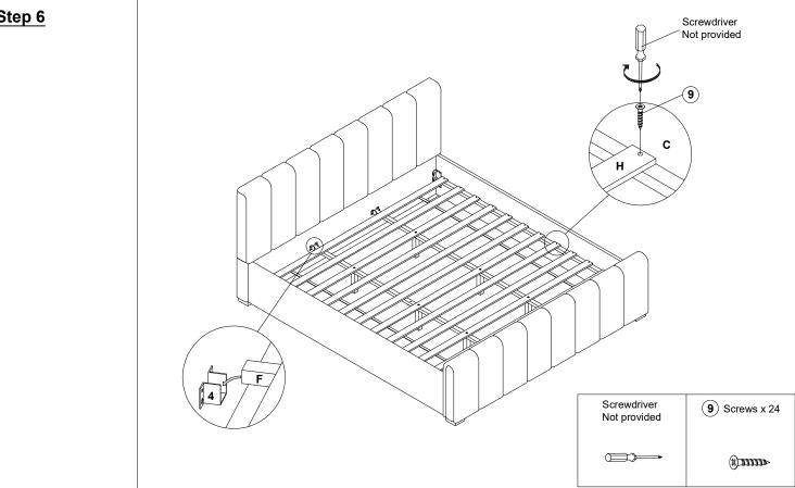
Fix the slats completed (H/F/G) the side rail (C) using screws (9), by screwdriver ( Not provided ) Secure the middle support bar (F) to the U-bracket (4)
