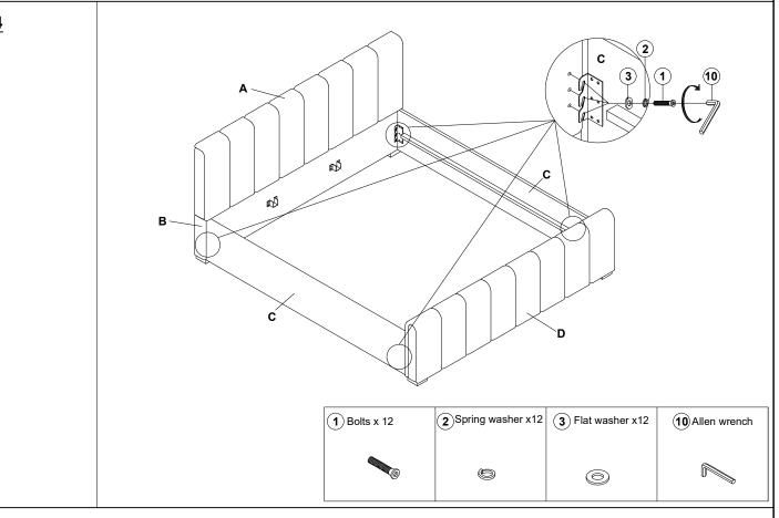
Fix the side rail (C) to the headboard (A/B) and the footboard (D) using bolts (1), spring washers (2) and Flat washers (3) by using Allen wrench (10)
