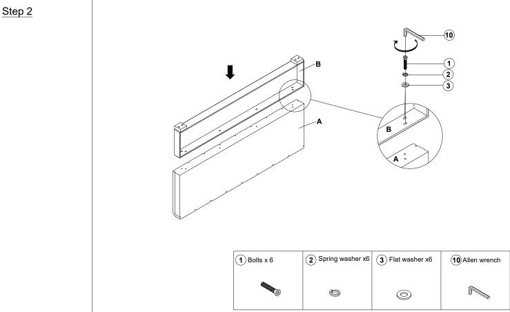
Fix the headboard below (B) to the headboard (A) using bolts (1), spring washers (2) and Flat washers (3) by using allen wrench (10)
