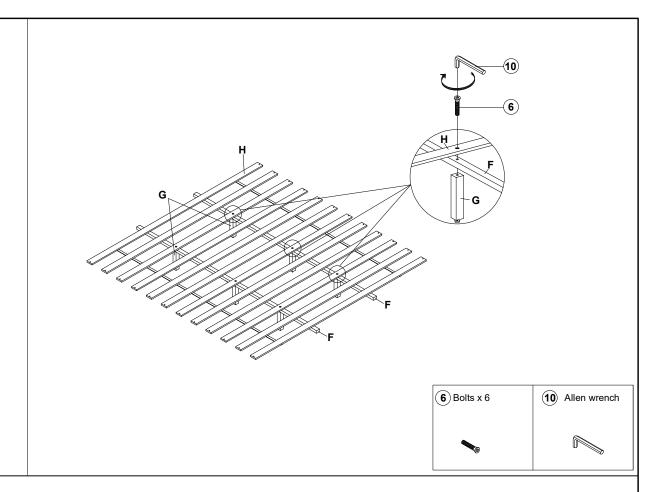
Fix the middle support legs (G) to middle support bar (F) and the slats (H) using bolts (6), by using allen wrench (10).
