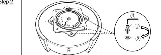
Place the chair base (B) on a soft, level surface. Position the swivel plate (C) on top, aligning its four slots. Secure them using the bolt (1), flat washer ring (2), and tighten with the allen key (3).
