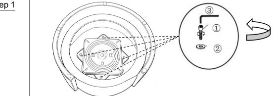
Please use the Allen wrench (③) to loosen the bolt (①) and flat washer (2), and remove the swivel plate (C) assembled under the chair base (B).
