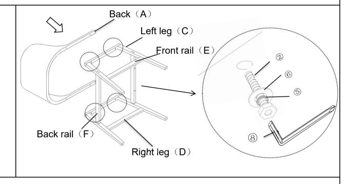
Attach the Legs(C+D) into the mounting positions of the Back(A) using Bolts(②), Spring Washer(⑤) and Washer(⑥) with Allen Wrench(⑧). Do not fully tighten the Bolts.
