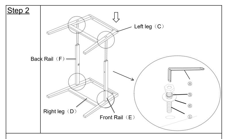
Attach the Legs(C+D) into the mounting positions of the Rails(E+F) using Bolts(1) Spring Washer(5) and Washer(6) with Allen Wrench(8). Do not fully tighten the Bolts.
