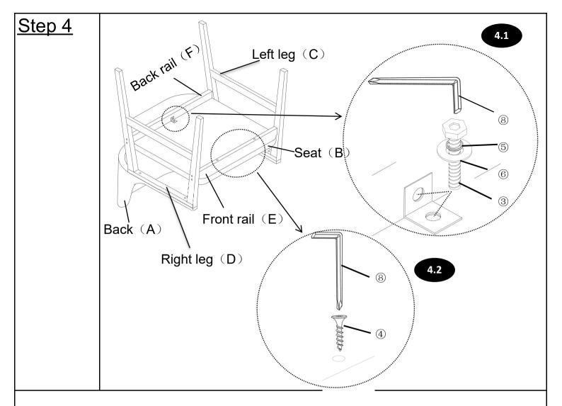
4.1)Attach the Back rail(F) and Seat(B) into the mounting positions of the angle iron( $\Im$ ) using Bolts( $\Im$ ),Spring Washer( $\Im$ ) and Washer( $\Im$ ) with Allen Wrench( $\Im$ ). Do not fully tighten the Bolts.
