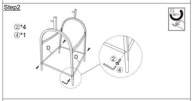
Attach the Pedal (D) to Left Leg (A) and Right Leg (B) using the Bolt (②) with Allen Wrench (④) as shown above.
