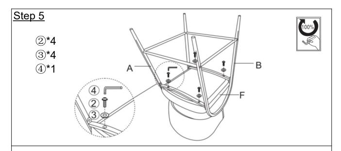
Place the Frame down on the edge of a clean, non-marring table top. Attach the Seat (F) to the Connection Rod (C) using the Bolts (②) and Washers (③) with the Allen Wrench (④)as pictured above.
