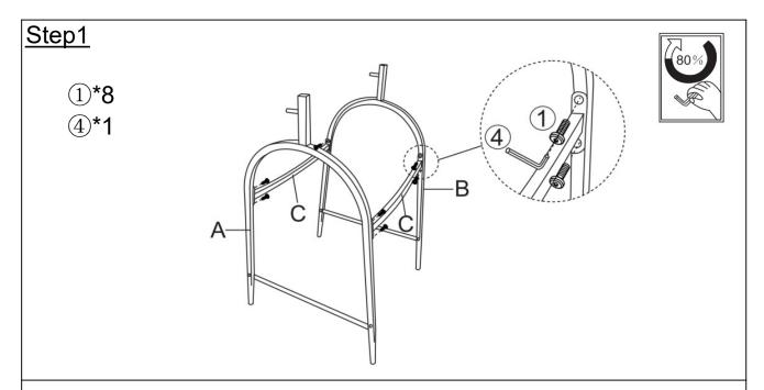
Attach the Connection Rod (C) to Left Leg (A) and Right Leg (B) using the Bolt (1) with Allen Wrench (4) as shown above.
