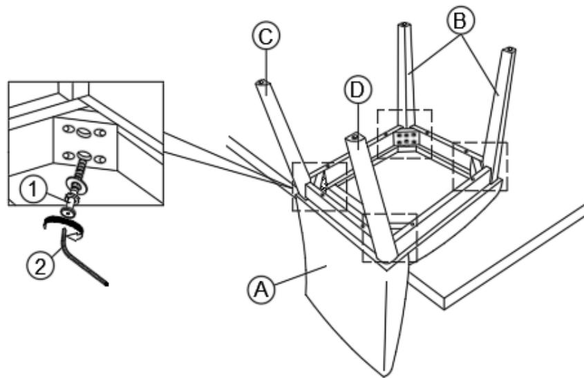
Assemble the Front Leg (B), Back Leg L(C) & R(D) to the Chair Body (A) using Bolt(①) with Allen Wrench(②).
