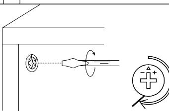
To tighten the Cam Lock, turn it clockwise on half
