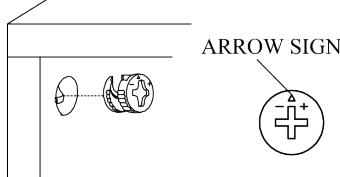
Insert the Cam Lock so the side opening fits over
