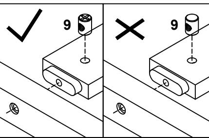
Note: Part 9 will face up with the "x" mark on it, otherwise it cannot be tightened
