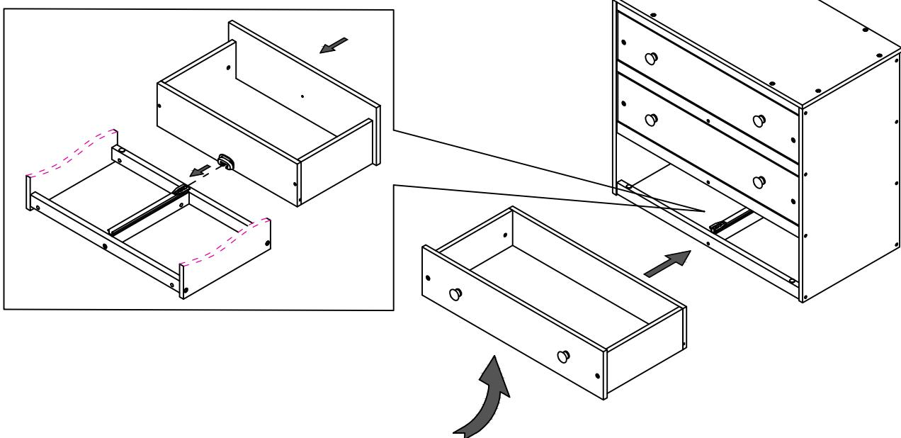
Align the slide rail at the bottom of the drawer and ensure it is secure, then push the drawer in firmly to make the slide rails smoothly on the track.
