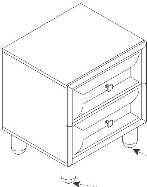
Note: Turn the feet adjusters to level up the unit.
