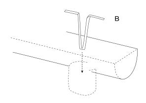
Hook Rain Chain (B) onto Gutter Clip (A). Wait for rain and enjoy! STEP 3 Note: Use a filter screen to prevent leaves and debris from dropping into your rain chain if needed.
