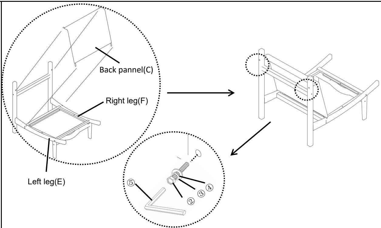
4.1) Slot the Back pannel(C) into the position holes on the Legs(E+F).
