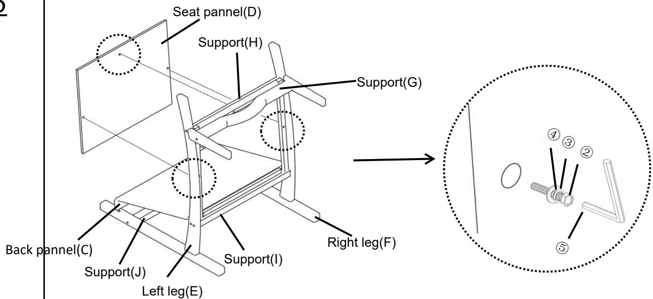
Attach the Seat pannel(D) into the Support(H) and Legs(E+F) using bolts(②),Spring washer(③) and Washer(④) with Allen wrench(⑤).
