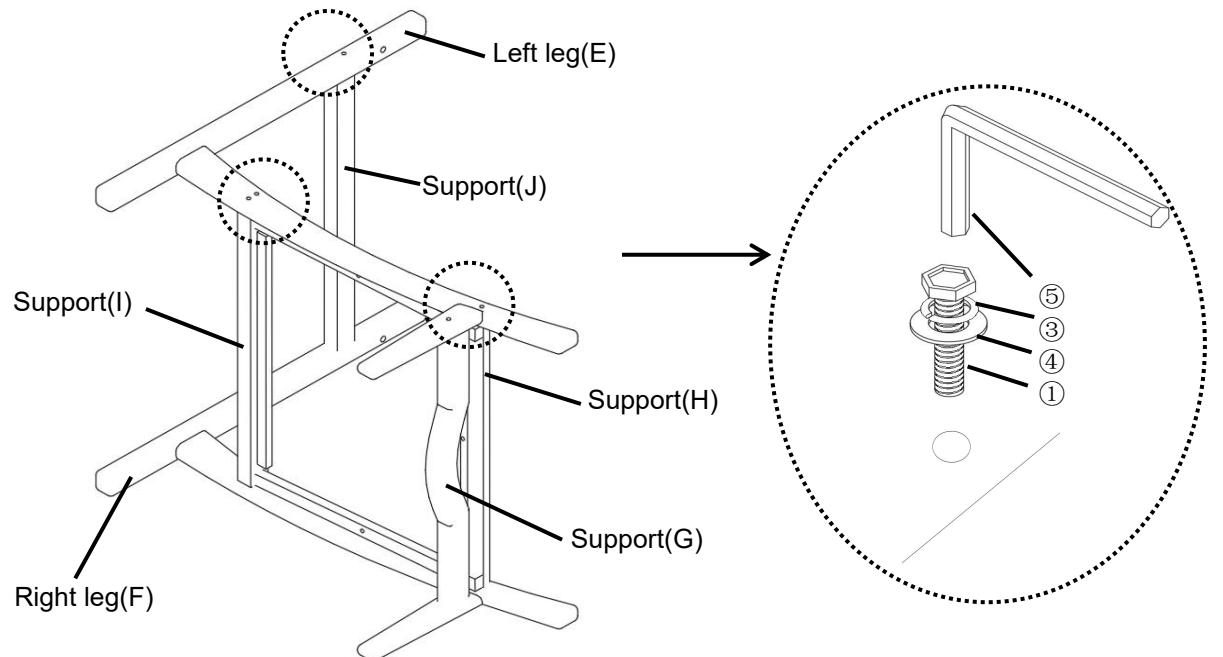
Attach the Leg(E+F) into the Supports(G+H+I+J) using bolts(①),Spring washer(③) and Washer(④) with Allen wrench(⑤).
