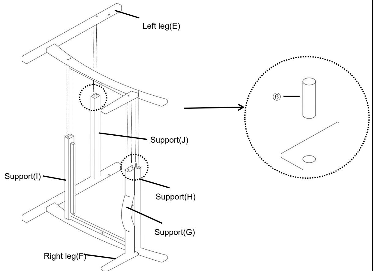
Slot the Wood plugs(⑥) into the mounting positons of the Support(G+H+J) and slot another end of the Wood plugs(⑥) into the Legs(E+F),as shown in picture.
