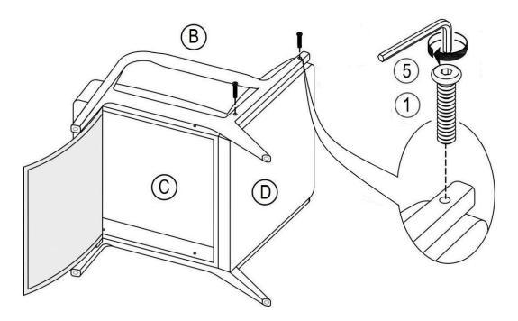
Do not fully tighten screws/ bolts until completely assembled
