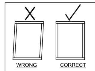
NB: Before tightening the plastic buckles and screws, please ensure the frame is square
