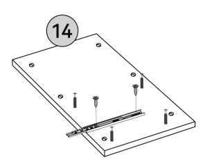
Lock with 3.5x12 self-correcting screws
