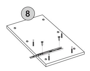
Lock with 3.5x12 self-correcting screws
