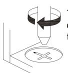
Turn cam lock clockwise to tighten.
