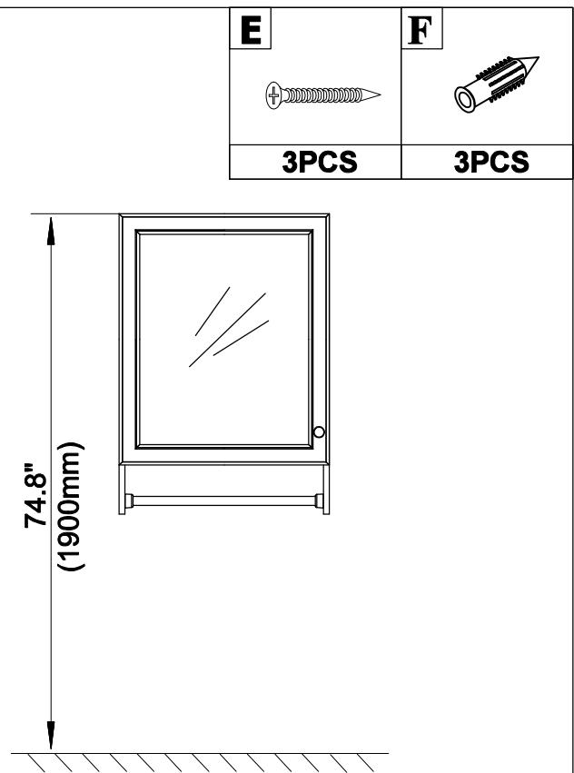
Draw the spacing between the walls and the No.6, punch holes in the wall, and fix the No.6 to the wall with screws.
