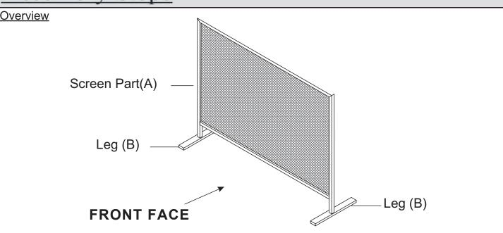
This Fireplace Screen has multiple parts and may require up to 10 minutes to assemble. To give you an overview of the Fireplace Screen parts, the above picture is to help you put the various parts into perspective. Please read through the instructions below to familiarise yourself with the parts and steps before assembly.
