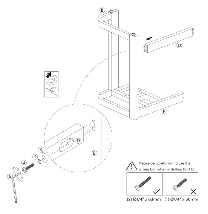
Now, assemble the Leg Frame Sub-Assembly (Left) (A) onto the other end of Footrest (D) and Cushion Support Frame Assembly (E) using the Hex Button Head Bolts (2), Spring Washers (4), and Half-moon Washers (3). Tighten with the Allen Key (6).
