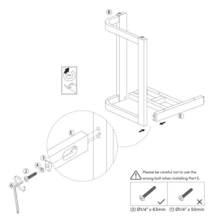
Install the Footrest (D) onto the Leg Frame Sub-Assembly (Right) (B) using the Hex Button Head Bolt (2), Spring Washer (4), and Half-moon Washer (3). Tighten firmly with the Allen Key (6).
