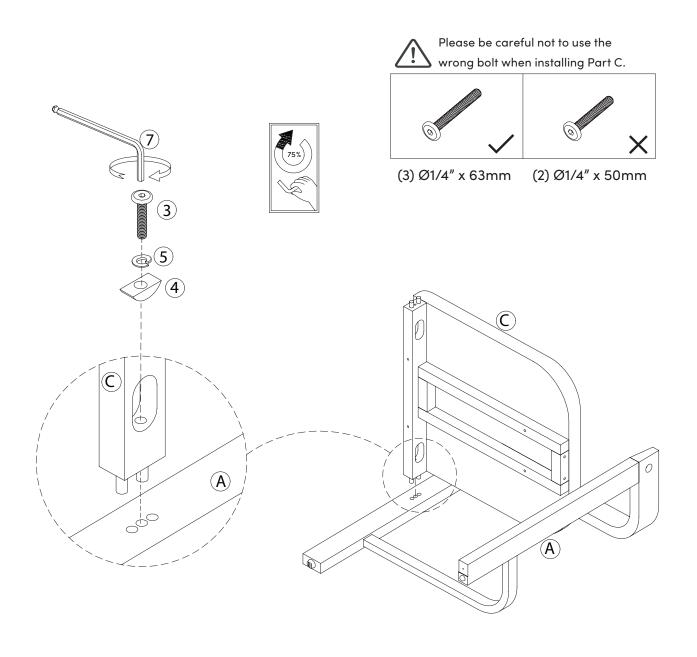
Now, assemble the Leg Frame Sub-Assembly (Right) (B) onto the other end of the Seat Cushion + Frame Assembly (C) using the Hex Button Head Bolt (3), Spring Washer (5), and Half-moon Washer (4). Tighten with the Allen Key (7).
