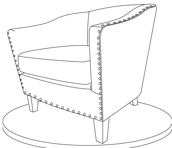
Place the chair on a LEVEL SURFACE to see if it wobbles. If it wobbles, press firmly down on both armrests at the same time. This will help to ensure all Bolts and gaps reach full alignment status. If no wobbles found, proceed to tighten all the Bolts. DO NOT fully tighten a BOLT in one go and then move on to the next. Rather, in a sequential manner, gradually tighten each Bolt until all Bolts are evenly secured. This methodology will ensure maximum evenness once all Bolts are fully tightened.
