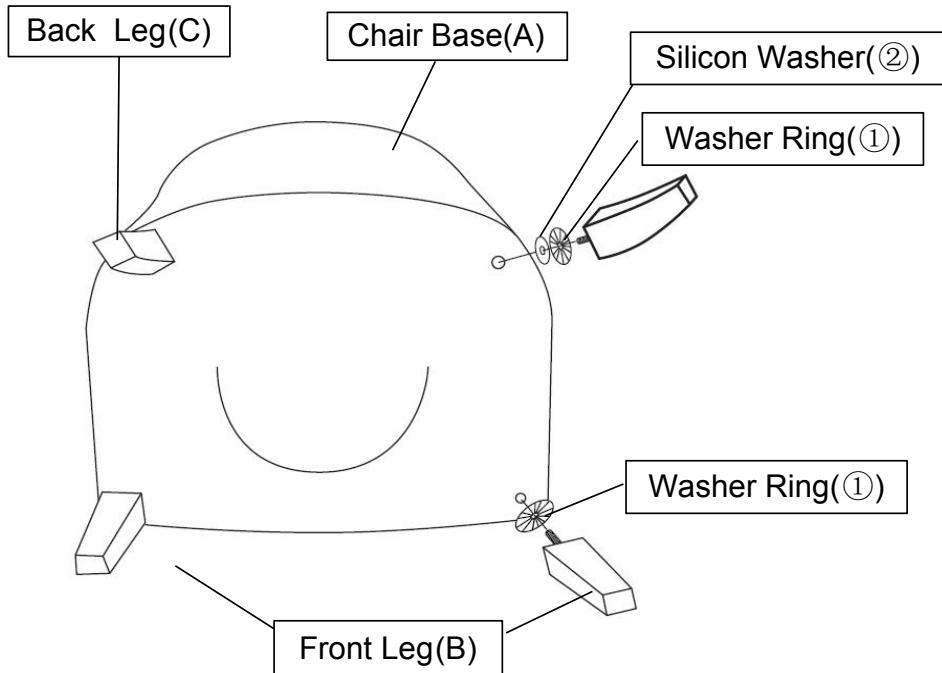
Install the Leg(B) into the bottom of the Chair Base(A) by placing the Washer Ring(①) onto the threaded stem. And then insert the threaded Stem into the threaded Mounting Position at each Corner of the Bottom of the Chair.
