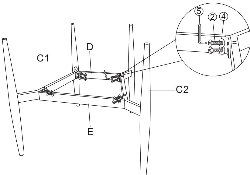
Attach the Back Connection Rod (D) and Front Connection Rod (E) to L leg(C1) and R Leg(C2) using the Washer (④),Bolt (②) with Allen Wrench (⑤) as pictured above.
