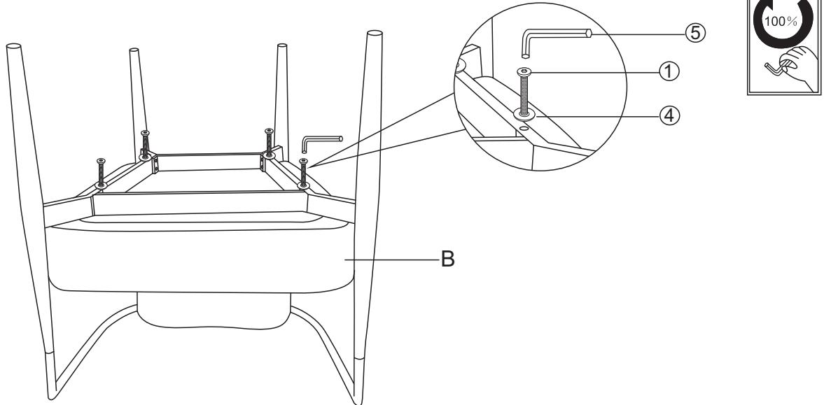
Attach the Seat Cushion (B) to the frame using Washer (4), Bolt (1) with Allen Wrench (5) as pictured above.
