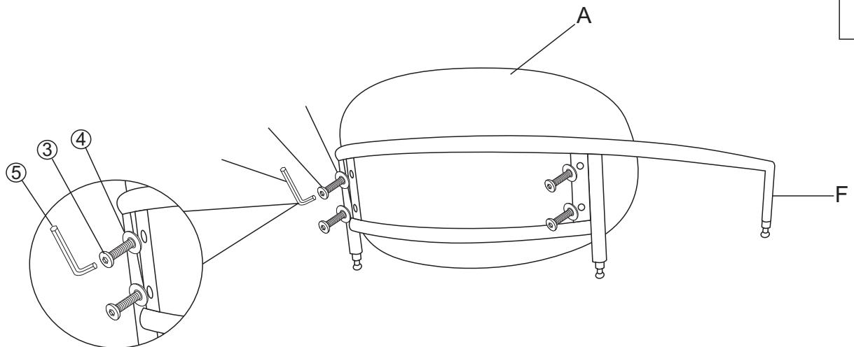
Attach the Back (A) to theBack Frame(F) using the Washer(④), Bolt (③) with Allen Wrench (⑤) as pictured above.
