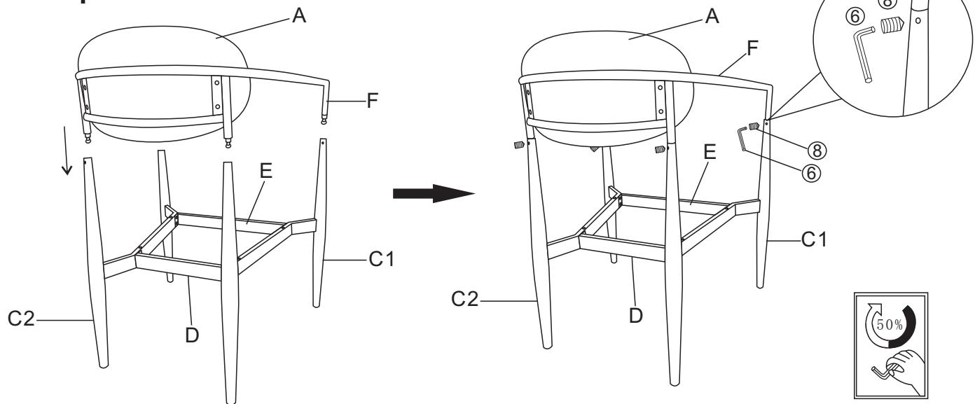
Attach the assembled back frame with Leg frame using Threaded Rod (8) with Allen Wrench (6) as pictured above.
