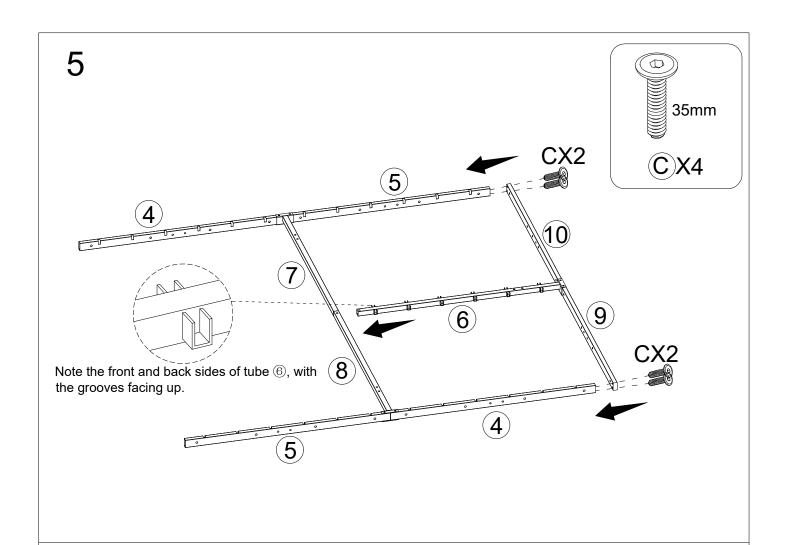
Note that the screws will not be installed in this step. After placing the accessory here, proceed to the next step on the next page
