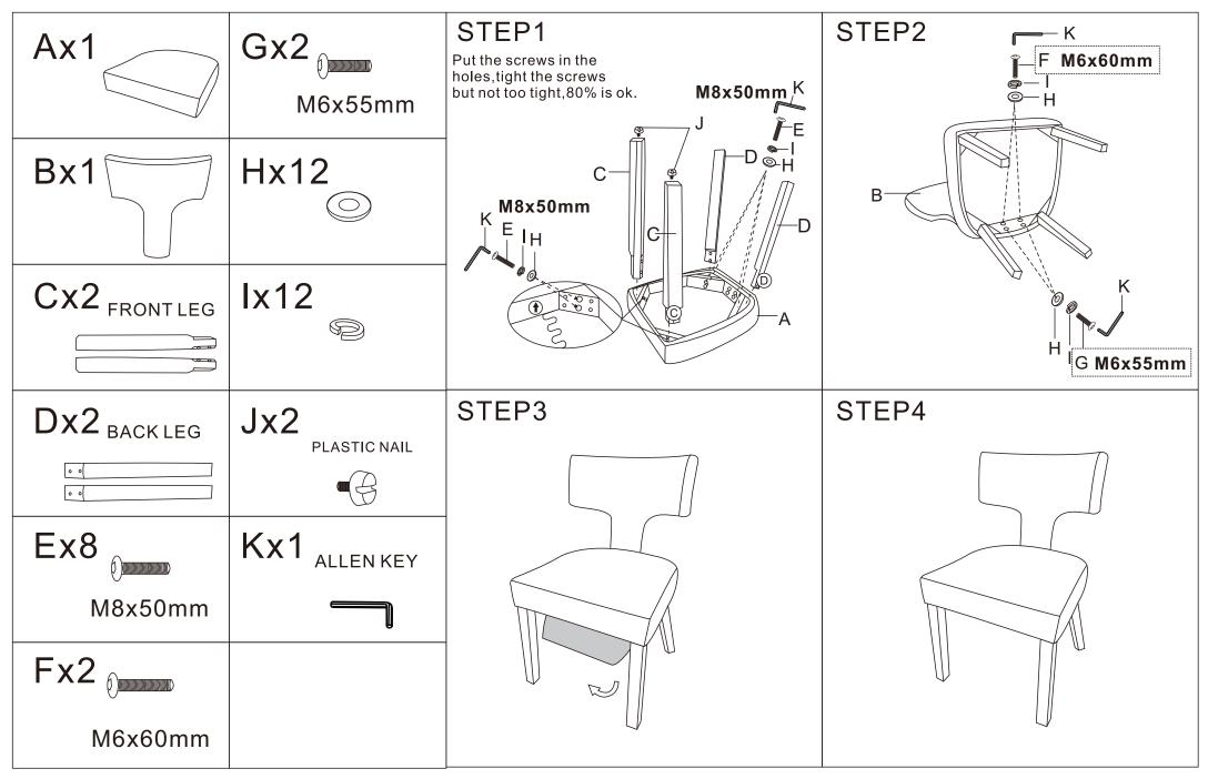
Notes:compare the length of each of screw, twist them to 80% instead of 100%; adjust the balance of the chair after installation, twist each screw tightly step by step.
