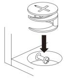
head should be in the centre of the cam lock when the two panels are joined.
