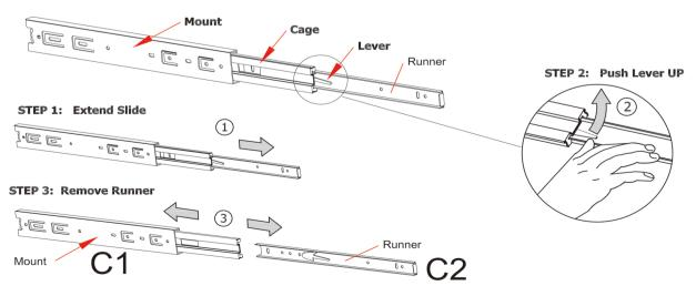
The guide rail needs to be divided into two parts: C1 and C2.
