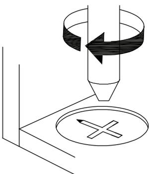
**EN\_**Turn cam lock clockwise to tighten.
