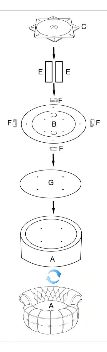
Step 1: Remove the fixed metal rotating disk screw and carefully extract it from the sofa base.
