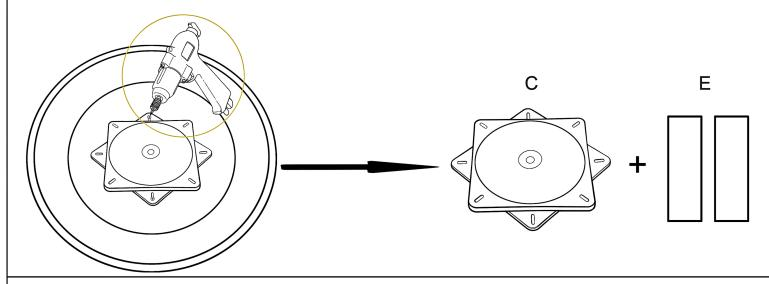
Step 2: Position two wooden boards at the bottom of the metal rotating disk, then securely attach the disk to the opposite plane of the sofa base using screws.
