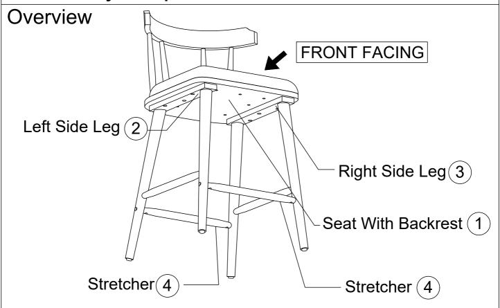
This Windsor stool has multiple parts and may require up to 30 minutes to assemble. To give you an overview of the Windsor stool parts, the above picture is to help you put the various parts into perspective. Please read through the instructions below to familiarize yourself with the parts and steps before assembly.
