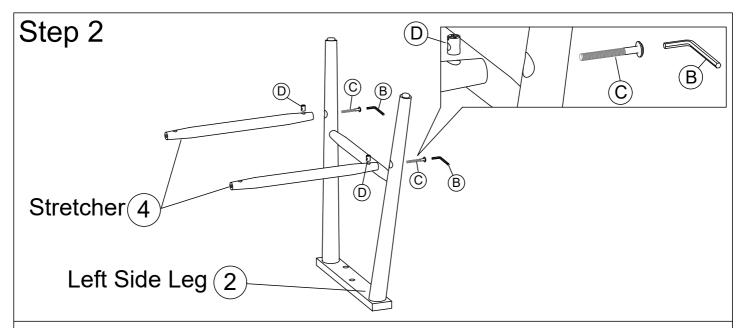
Place the Left Side Leg (2) on a clean, soft surface with the top side facing upward to prevent scratches or damage.
