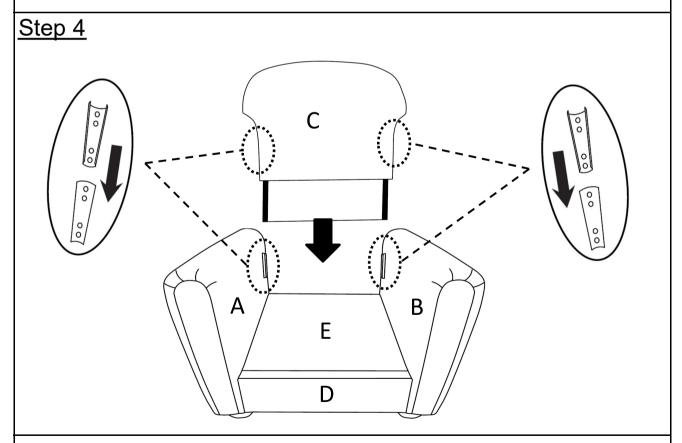
Attach the Back Frame (C) to the Left Arm (A) and the Right Arm(B).
