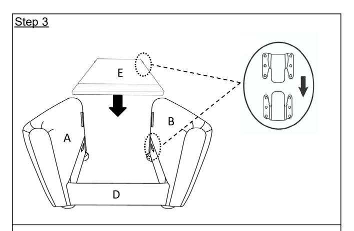
Insert the Seat Base(E) into the latch of the Left Arm(A) and the Right Arm(B).
