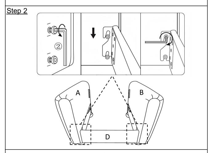
Tighten the Front Panel(D) with the Left Arm (A) and the Right Arm(B) By using Allen Wrench(②).
