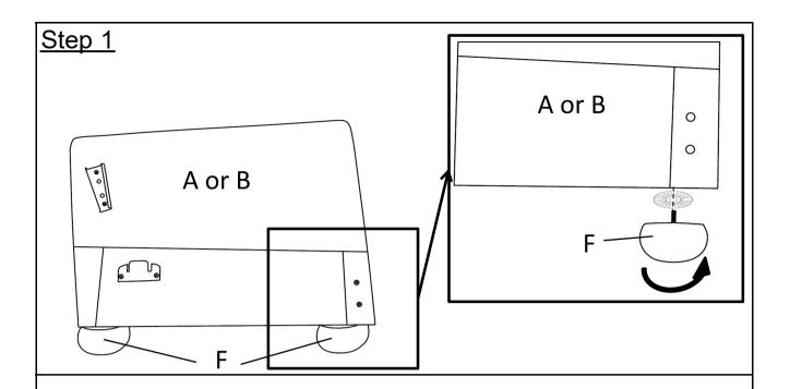
Screw Wooden Leg(F) with Plastic Washer(①) to both Left Arm(A) and Right Arm(B) as picture shows
